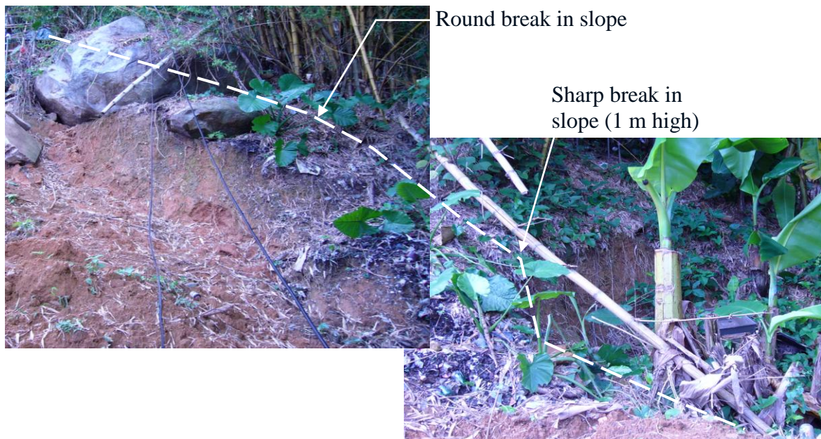
Plate 19 - Break in Slope on the Adjacent Hillside to the North of the Landslide (Photograph taken on 13 September 2005)
