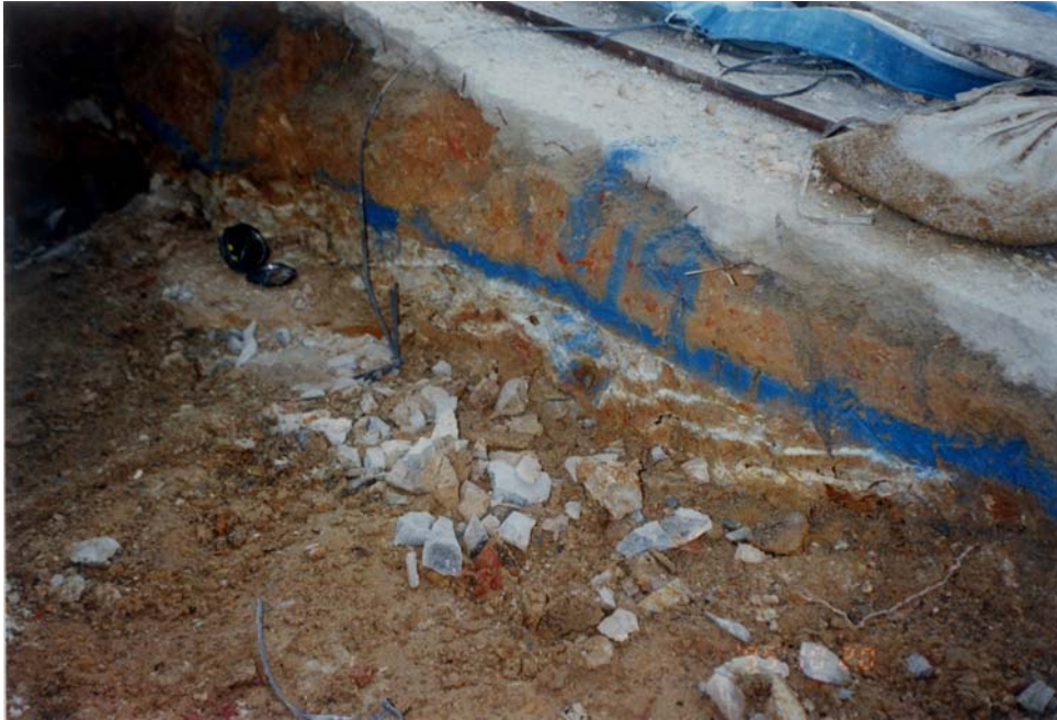
Plate 12 - Remnants of Kaolinite-rich Altered Tuff at the Western Toe of the Landslide (Photograph Taken on 20 October 1995. See Figure 21 for Location)
