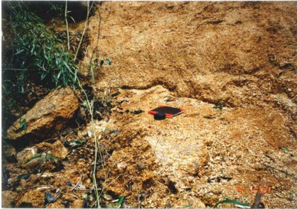
Plate 6 - A Joint Exposed in an Erosion Gully, Dipping at 30^{\circ} , Forming the Lower Part of the Rupture Surface (Photograph Taken on 4 August 1997. See Figure 14 for the Location)
