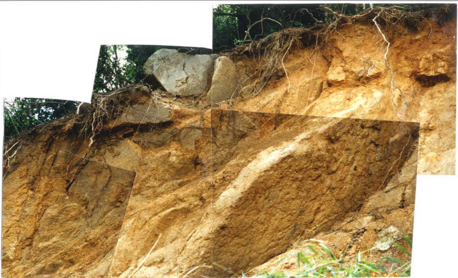
Plate 3 - View of Southwest Flank of the Landslide (Photograph Taken on 7 July 1997. See Figure 14 for Location. Note the Grey Decomposed Granite Boulder on the Ground Surface and the Vertical Planar Discontinuity in the Lower Right Corner of the Photograph Associated with a Dominant Set of Sub-Vertical Veins and Joints)
