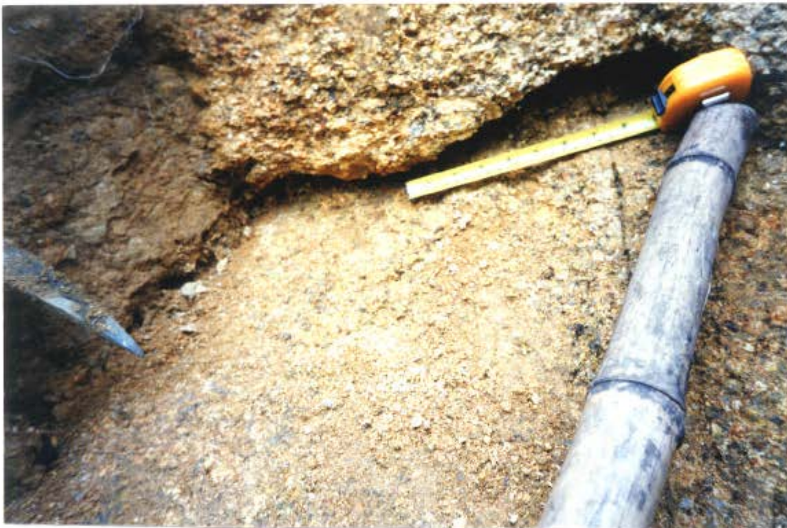
Plate 9 - View of an Erosion Pipe in the Northeast Corner of the Main Scarp (Photograph Taken on 23 September 1997. See Figure 14 for Location)
