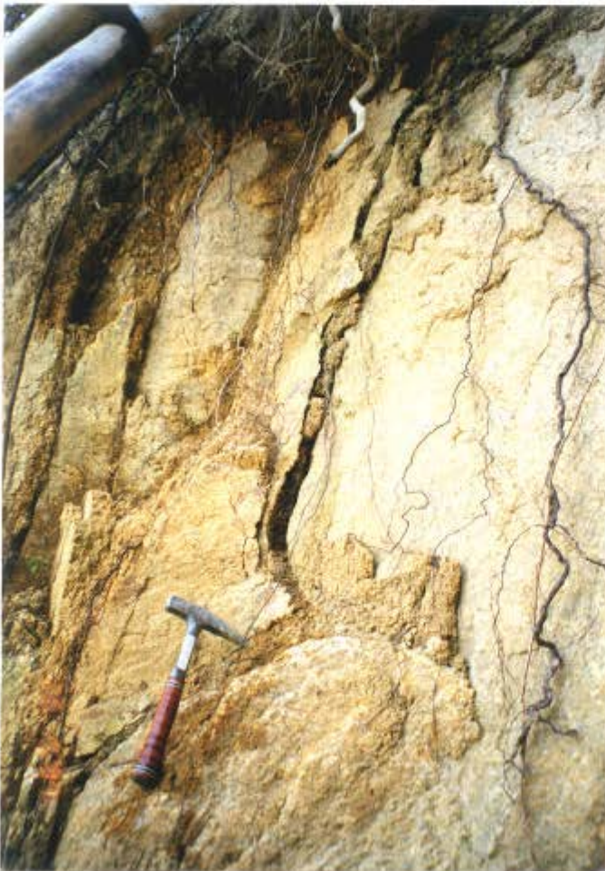
Plate 6 - A Joint Exposed in an Erosion Gully, Dipping at 30^{\circ} , Forming the Lower Part of the Rupture Surface (Photograph Taken on 4 August 1997. See Figure 14 for the Location)
