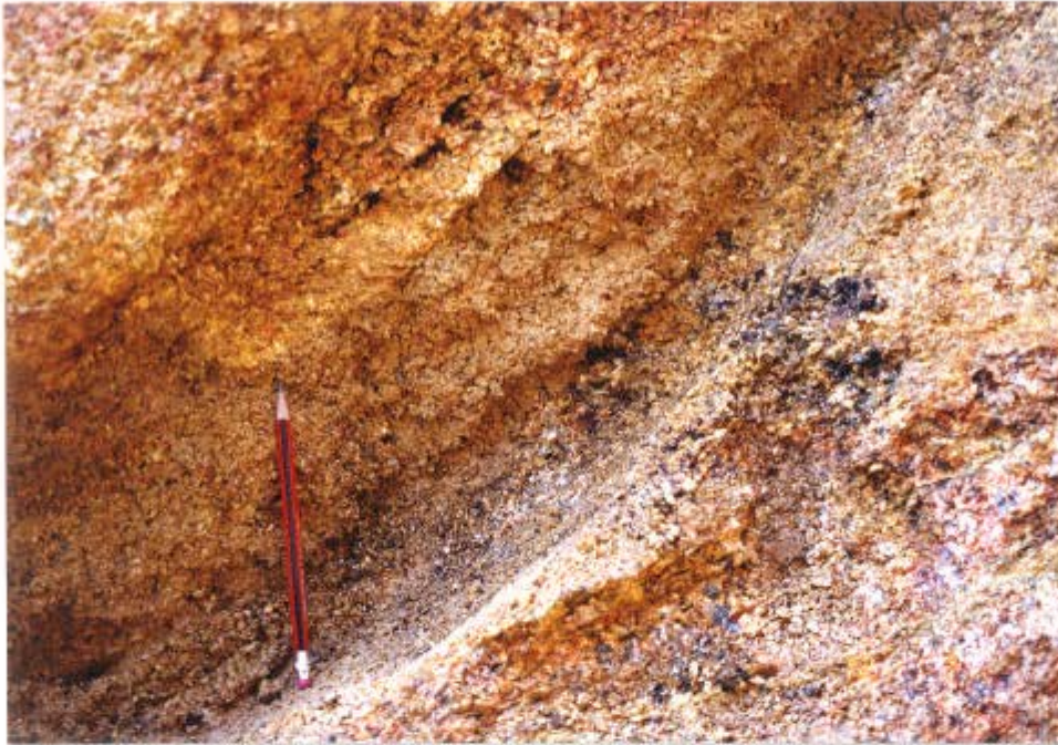
Plate 8 - Layer of Sheared Material at the Base of the Landslide (Photograph Taken on 12 November 1997. Note the Layer is about as Thick as the Length of Pencil. See Figure 14 for Location)
