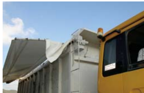
配備機動蓋掩的卸泥車 Dump truck with mechanical truck cover
