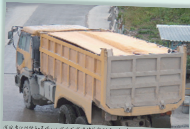
運泥車使用機動蓋，以減低在運送建築廢料時所散發的泥塵 Use of mechanical covers on trucks for dust control during transportation of construction waste
