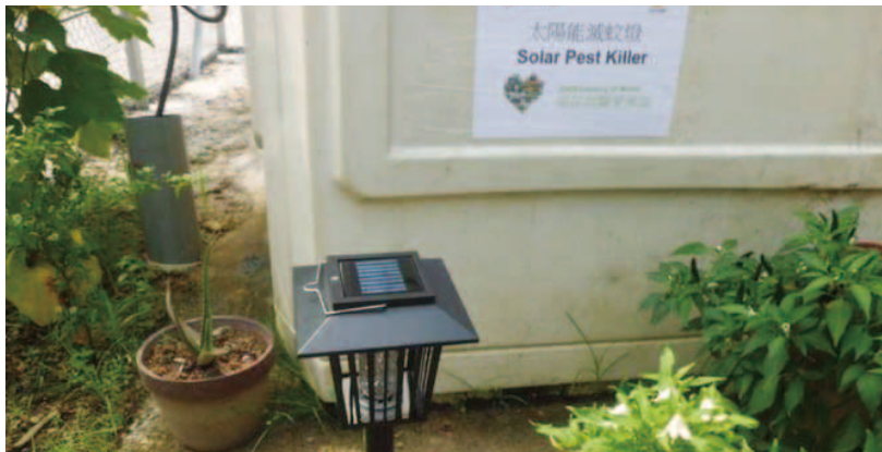
蓮塘 / 香園圍口岸 Liantang/Heung Yuen Wai Boundary Control Point 太陽能滅蚊燈防止蚊子滋生 Solar pest killer for prevention of mosquito breeding
