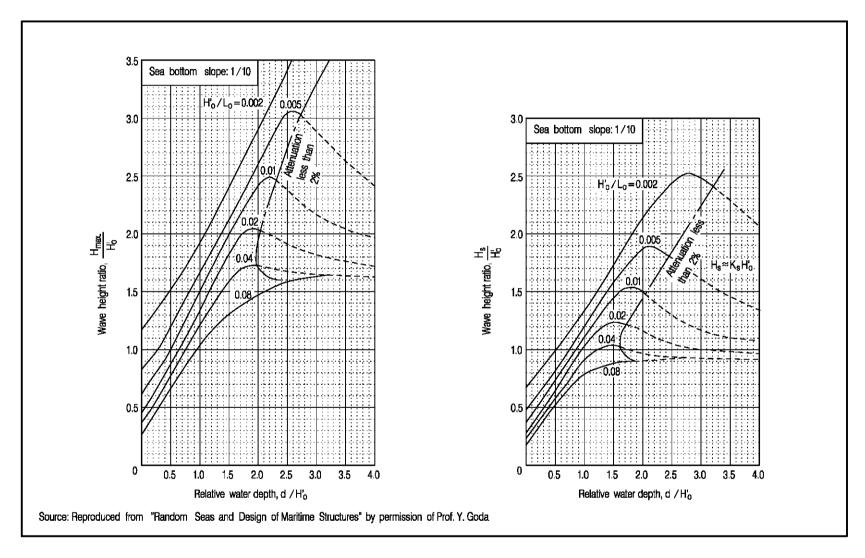
Figure A2 - Estimation of Wave Height in the Surf Zone (Sheet 1 of 4)
