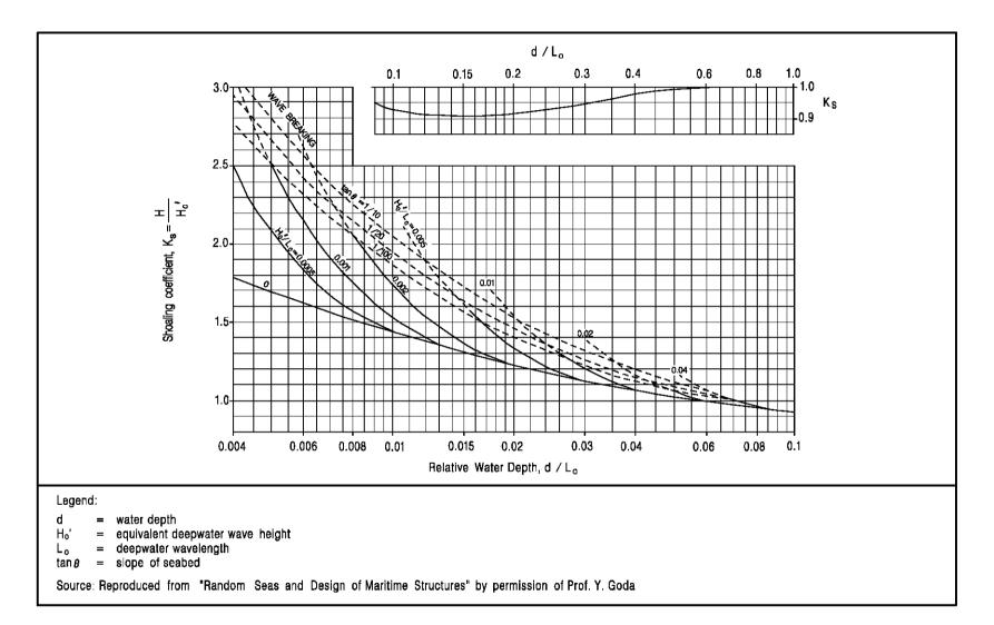
Figure A1 - Diagram of Nonlinear Wave Shoaling
