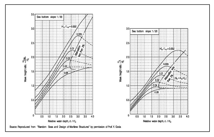
Figure A2 - Estimation of Wave Height in the Surf Zone (Sheet 2 of 4)
