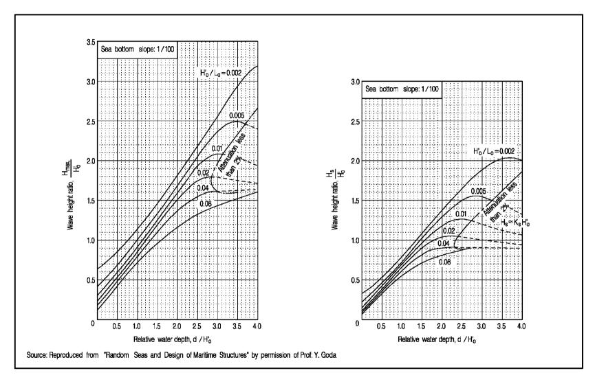
Figure A2 - Estimation of Wave Height in the Surf Zone (Sheet 4 of 4)
