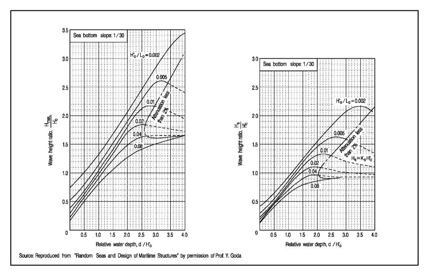
Figure A2 - Estimation of Wave Height in the Surf Zone (Sheet 3 of 4)
