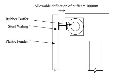
Load case 2: Berthing load at mid-span of steel waling
