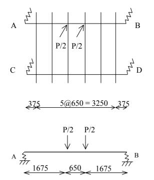
Assume that the total berthing energy is to be equally shared between two buffers (A and B). The total energy to be absorbed for accident loading should be at least 50% greater than that for normal loading.
