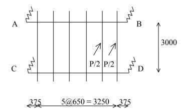
Similarly to load case 2, assume that the total berthing energy is equally shared between two buffers (B and D). Therefore, the reaction force at B = 600 kNBy symmetry, the reaction force at A = 600 kN and P/2 = 600 kN
