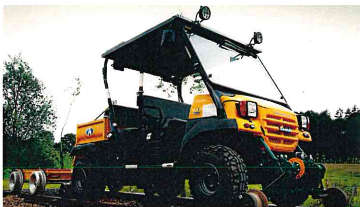
Plate 8.3 Typical Backup Access Vehicle (BAV)
