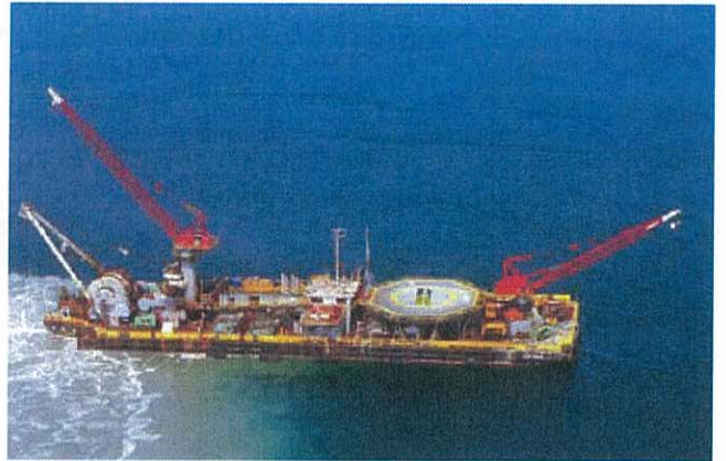
“Canyon Horizon” Pipe Jetting Barge (Horizon Offshore equipment)
