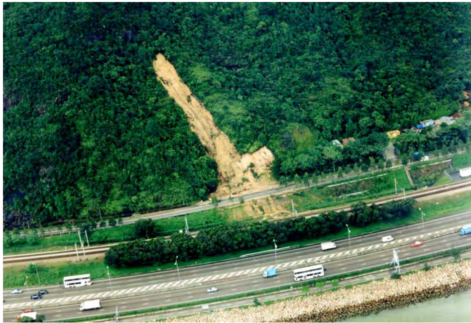
Plate 1.6 Open-slope Debris Avalanche on Natural Terrain in Ma Liu Shui in July 1997 (Lam, 1999)
