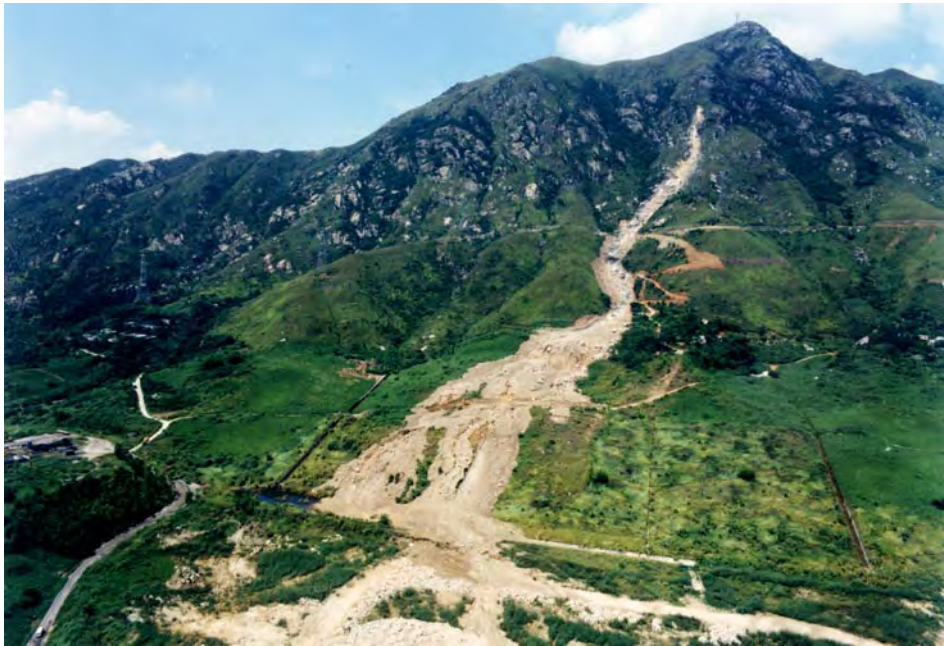
Plate 1.5 Large Channelised Debris Flow on Natural Terrain in Tsing Shan, near Tuen Mun, in September 1990 (King, 1996)
