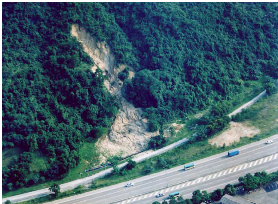
Plate 1.7 Open-slope Debris Avalanche on Natural Terrain in Ma On Shan in July 1997 (Halcrow, 1999b)
