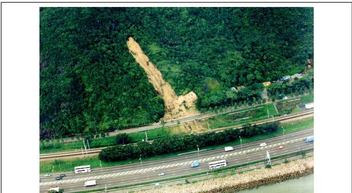
Plate 1.5 Large Channelised Debris Flow on Natural Terrain in Tsing Shan, near Tuen Mun, in September 1990 (King, 1996)
