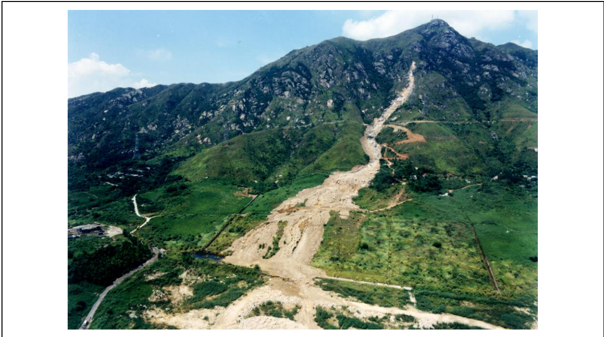
Plate 1.5 Large Channelised Debris Flow on Natural Terrain in Tsing Shan, near Tuen Mun, in September 1990 (King, 1996)
