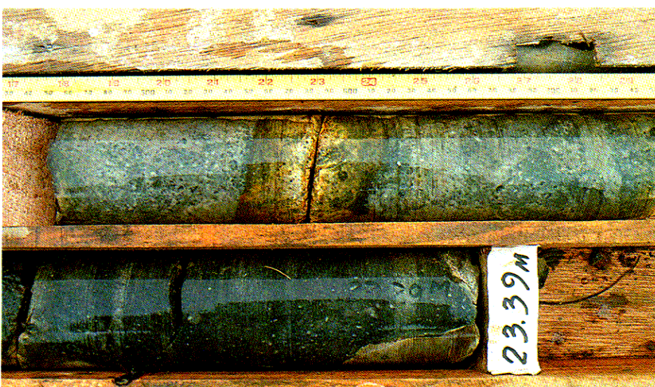
Plate 2.14 - Moderately Decomposed Seam (Grade III) in Slightly Decomposed Volcanic Rock (Grade II) : Detail H
