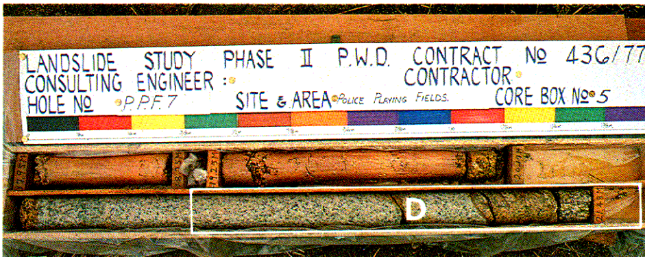
Plate 2.19 - Highly Decomposed Granite Rock (Grade IV), 17.95 to 20.17 m Slightly Decomposed Granite Rock (Grade II), 20.17 to 21.23 m Moderately Decomposed Granite Rock (Grade III), 21.23 to 21.48 m
