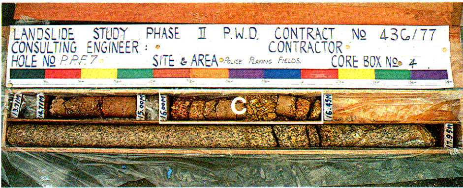
Plate 2.18 - Highly Decomposed Granite Rock (Grade IV), 13.71 to 16.45 m Moderately Decomposed Granite Rock (Grade III), 16.45 to 17.95 m
