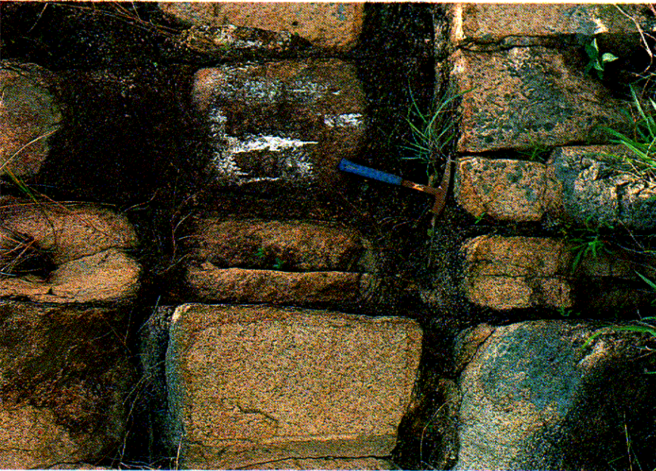
Plate 1.7 - Granite Showing Intense Weathering along Joints : Zone C
