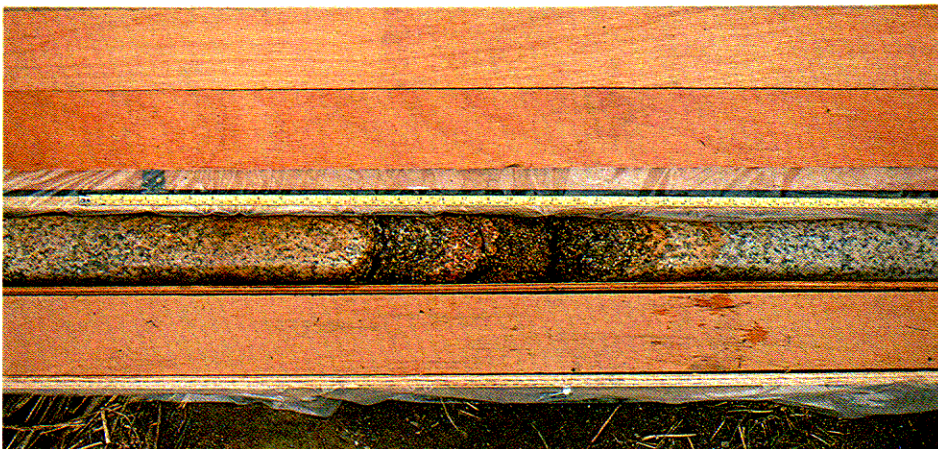
Plate 2.26 - Highly Decomposed Seam (Grade IV) in Slightly Decomposed Granite Rock (Grade II) : Detail E
