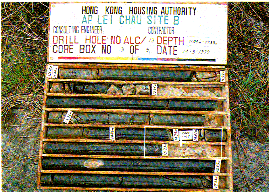
Plate 2.4 - Slightly Decomposed Volcanic Rock (Grade II), 11.04 to 17.33 m
