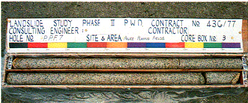
Plate 2.17 - Slightly Decomposed Granite Rock (Grade II), 10.71 to 13.71 m
