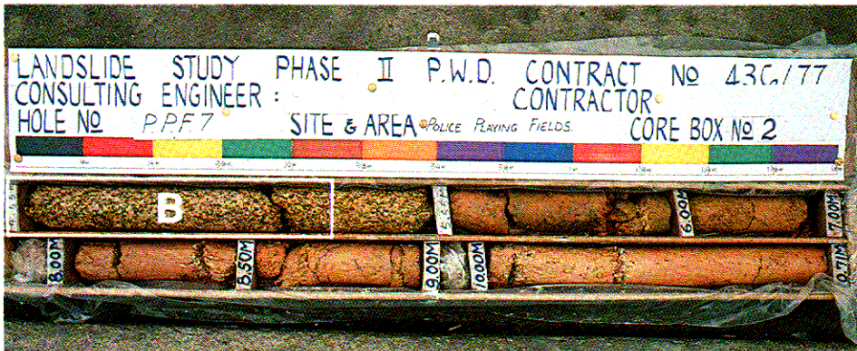
Plate 2.16 - Moderately Decomposed Granite Rock (Grade III), 4.65 to 5.55 m Highly Decomposed Granite Rock (Grade IV), 5.55 to 10.71 m
