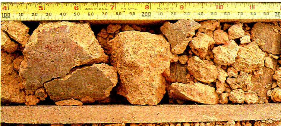
Plate 2.8 - Completely Decomposed Volcanic Rock (Grade V) : Detail B
