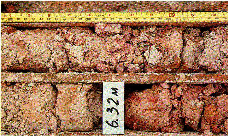
Plate 2.9 - Completely Decomposed Volcanic Rock (Grade V) : Detail C
