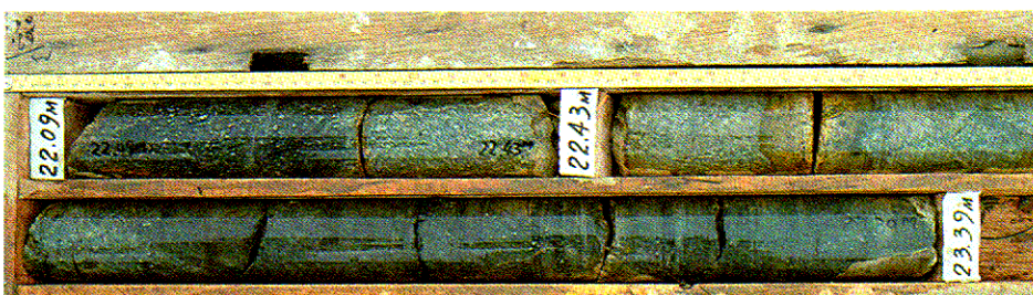
Plate 2.13 - Slightly Decomposed Volcanic Rock (Grade II) : Detail G
