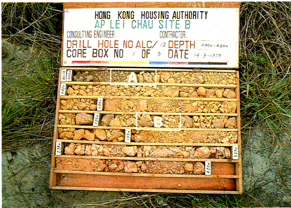
Plate 2.2 - Volcanic Residual Soil (Grade VI), 0 to 0.24 m Completely Decomposed Volcanic Rock (Grade V), 0.24 to 4.20 m
