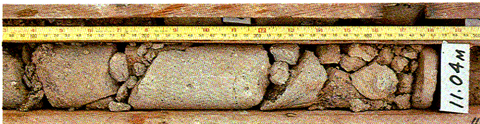
Plate 2.11 - Moderately Decomposed Volcanic Rock (Grade III) : Detail E
