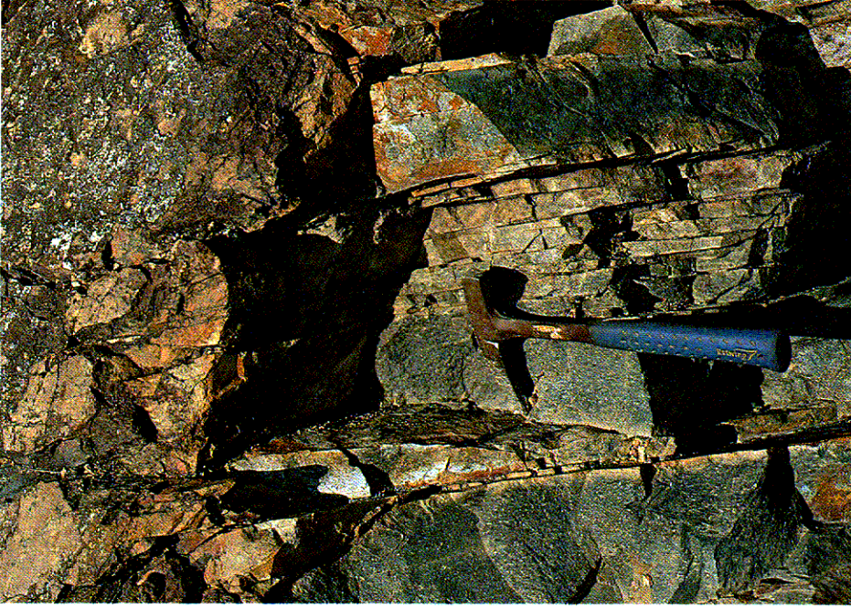
Plate 1.10 - Volcanic Rock with Staining along Joints : Zone D
