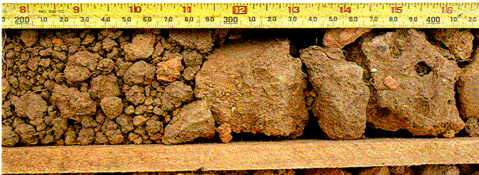
Plate 2.7 - Volcanic Residual Soil (Grade VI) : Detail A
