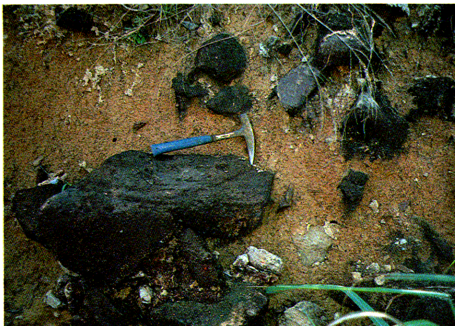
Plate 1.14 - Volcanic Colluvium Showing Boulders Contained in a Structureless Soil Matrix
