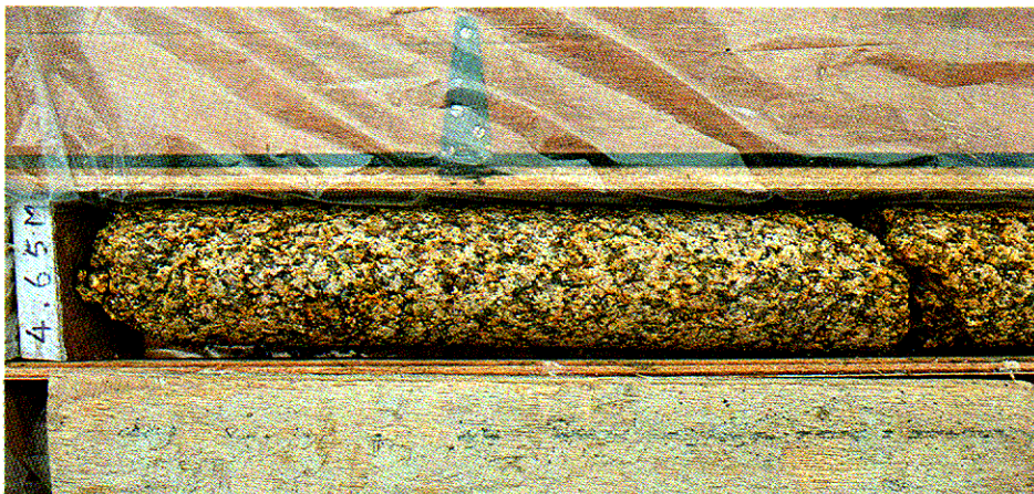
Plate 2.23 - Moderately Decomposed Granite Rock (Grade III) : Detail B
