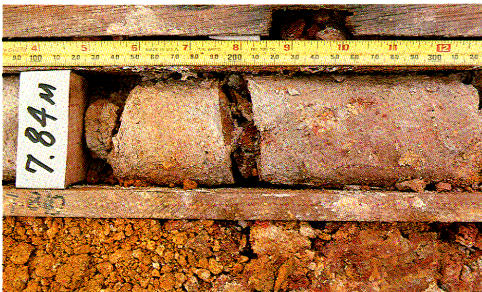
Plate 2.10 - Completely Decomposed Volcanic Rock (Grade V) with Stained Discontinuities : Detail D
