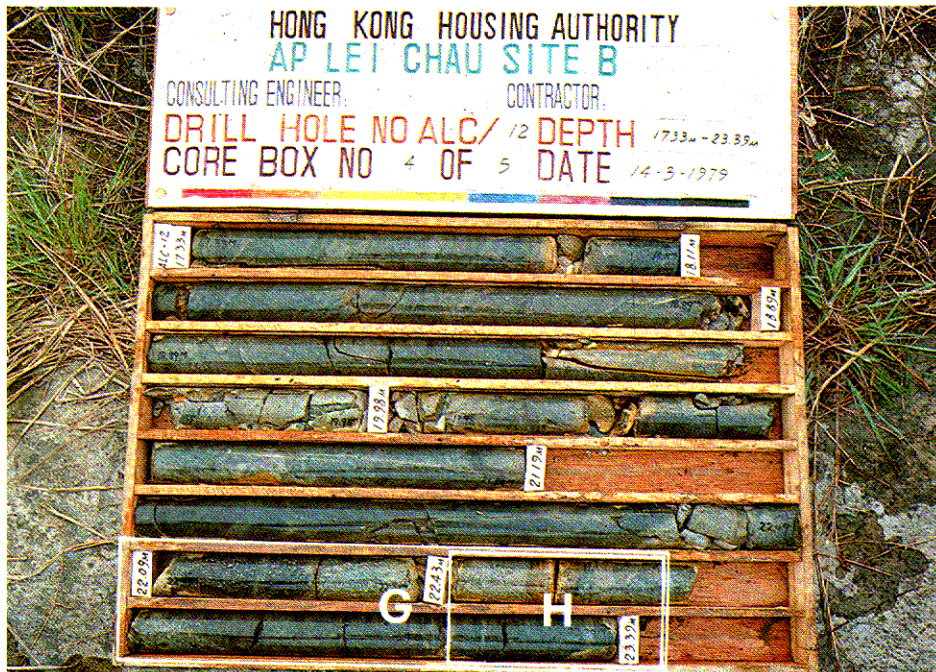
Plate 2.5 - Slightly Decomposed Volcanic Rock (Grade II), 17.33 to 23.39 m
