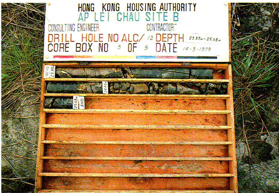
Plate 2.6 - Slightly Decomposed Volcanic Rock (Grade II), 23.39 to 25.08 m
