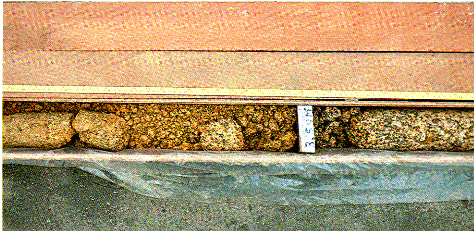
Plate 2.22 - Highly Decomposed Granite Rock (Grade IV) : Detail A
