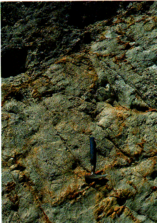
Plate 1.4 - Weathered Volcanic Rock in Zone B Showing Well-defined Relict Jointing
