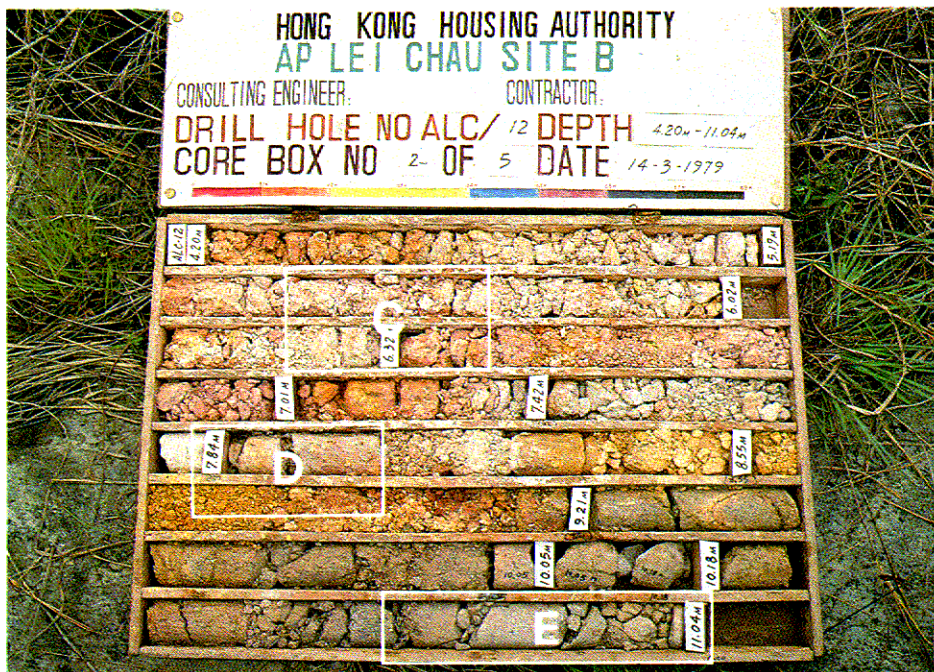
Plate 2.3 - Completely Decomposed Volcanic Rock (Grade V), 4.20 to 9.21 m Highly Decomposed Volcanic Rock (Grade IV), 9.21 to 10.05 m Moderately Decomposed Volcanic Rock (Grade III), 10.05 to 11.04 m
