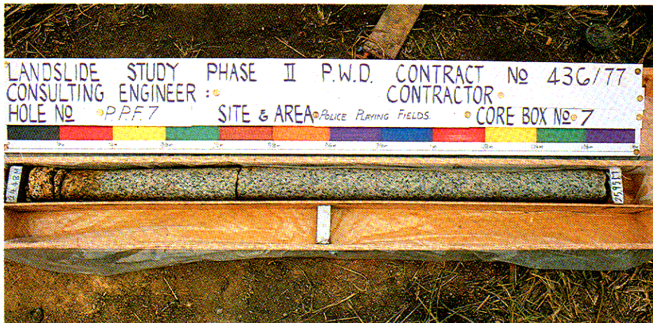
Plate 2.21 - Slightly Decomposed Granite Rock (Grade II), 24.48 to 25.95 m
