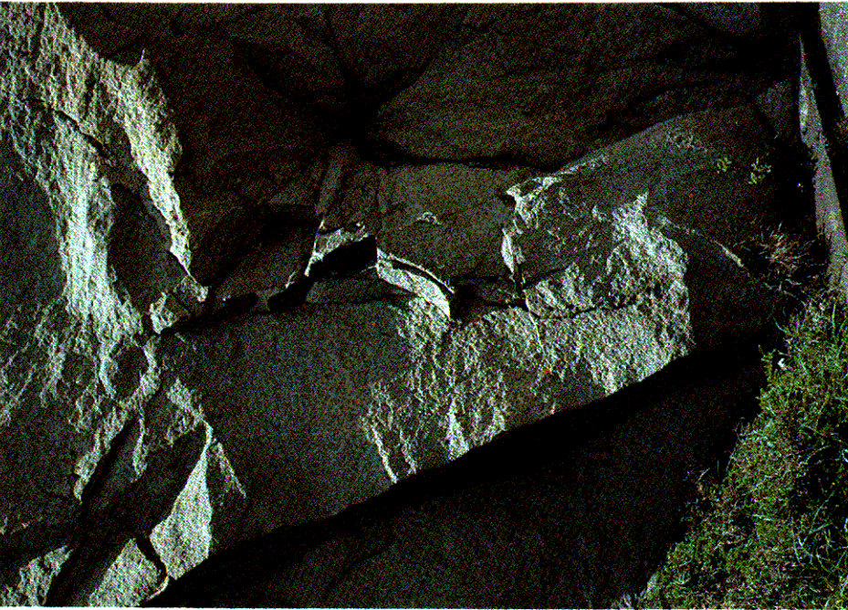
Plate 1.9 - Granite Showing Slight Staining on Joints : Blasting Fractures Can Be Seen at Centre Right : Zone D
