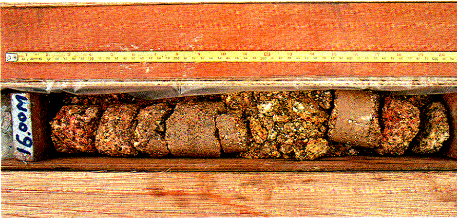
Plate 2.24 - Highly Decomposed Granite Rock (Grade IV) : Detail C
