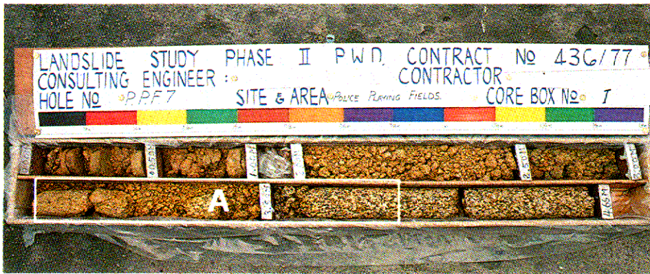
Plate 2.15 - Completely Decomposed Granite Rock (Grade V), 0 to 1.00 m Highly Decomposed Granite Rock (Grade IV), 1.00 to 3.59 m Moderately Decomposed Granite Rock (Grade III), 3.59 to 4.65 m
