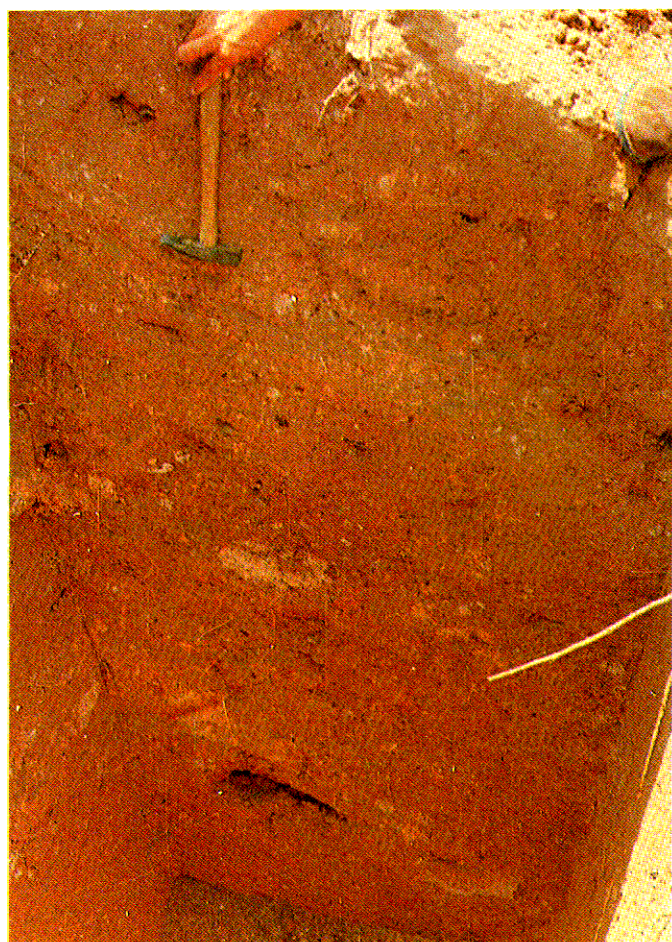
Plate 1.13 - Granitic Fill Showing Layering Parallel to the Slope
