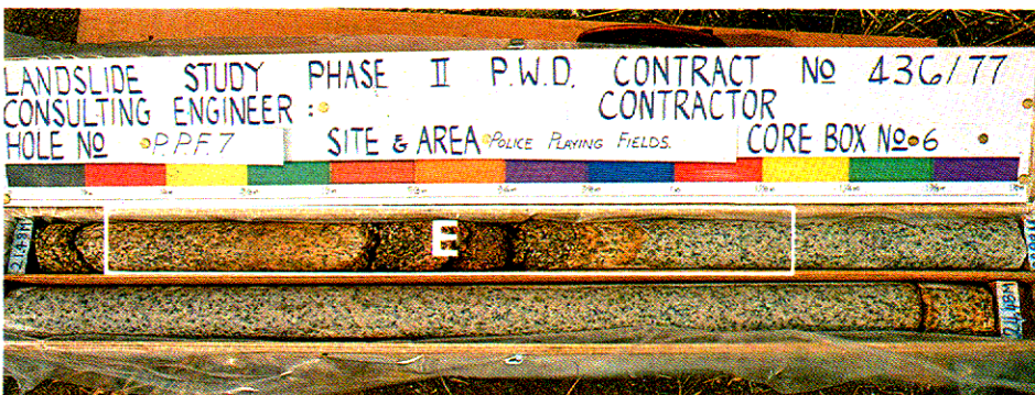
Plate 2.20 - Moderately Decomposed Granite Rock (Grade III), 21.48 to 22.00 m Slightly Decomposed Granite Rock (Grade II), 22.00 to 24.48 m
