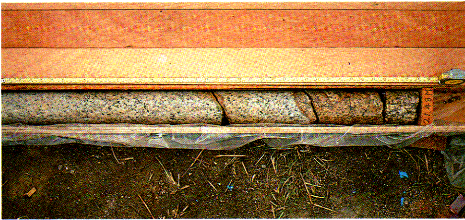
Plate 2.25 - Slightly Decomposed (Grade II) Becoming Moderately Decomposed Granite Rock (Grade III) : Detail D
