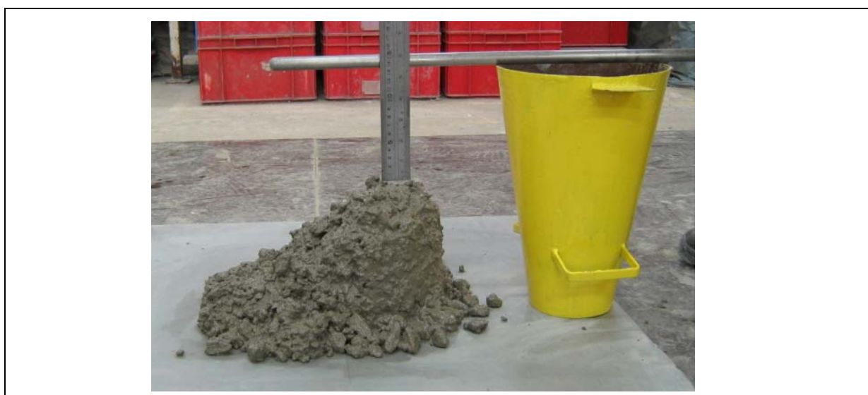
Figure 2 - Photograph of Shear Slump
