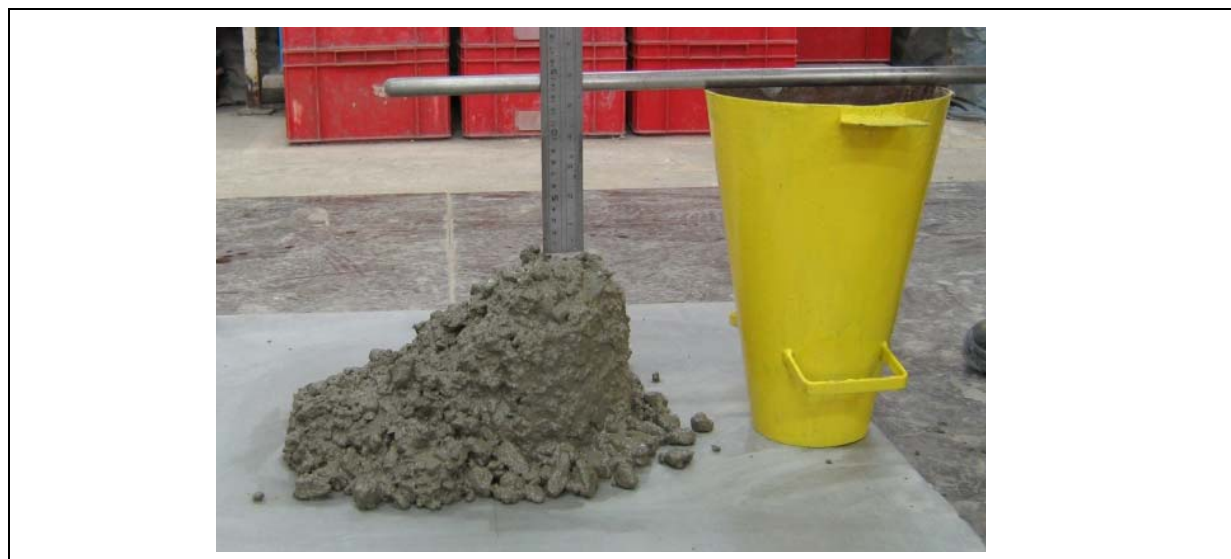
Figure 2 - Photograph of Shear Slump
