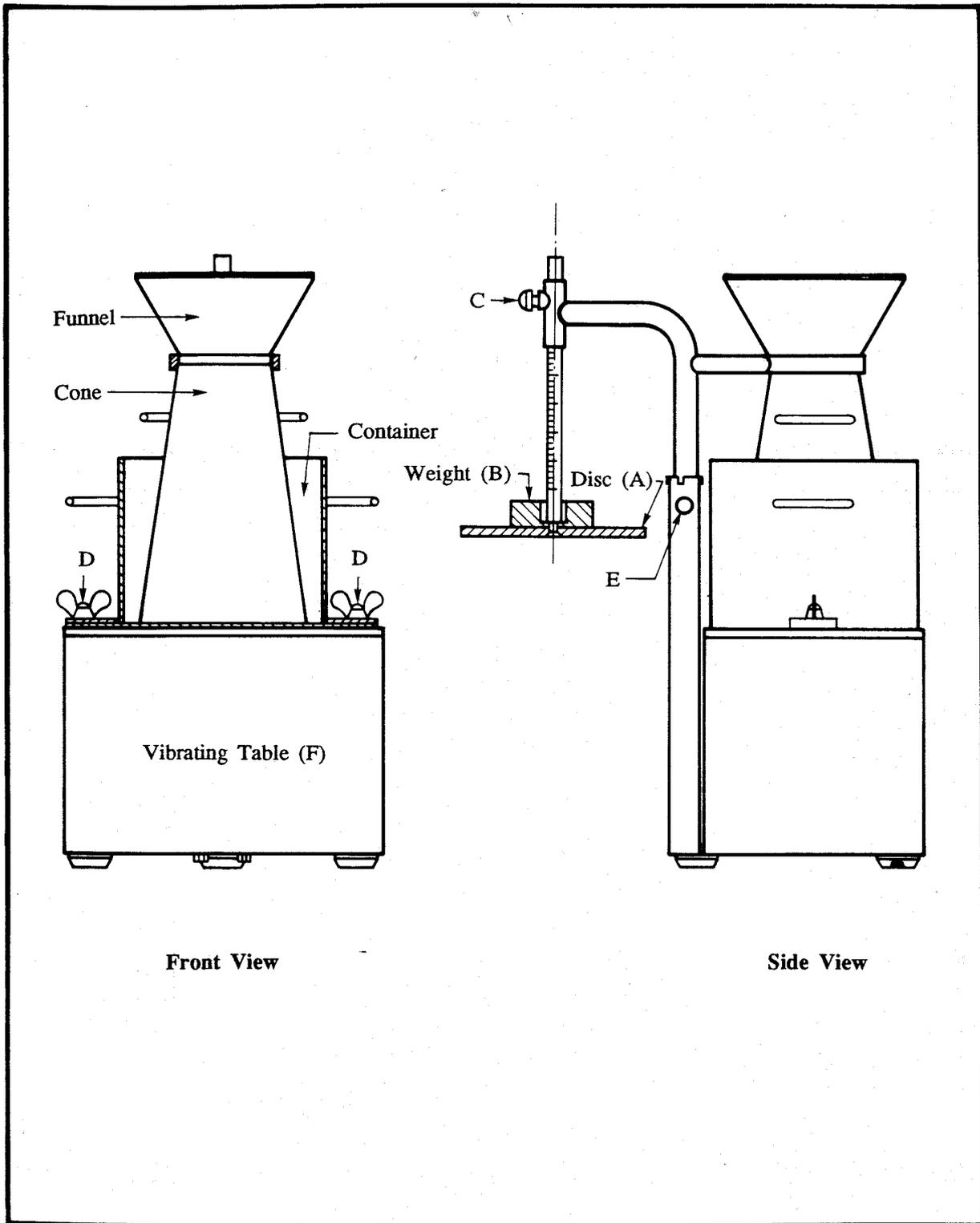
Figure 2 - Consistometer
