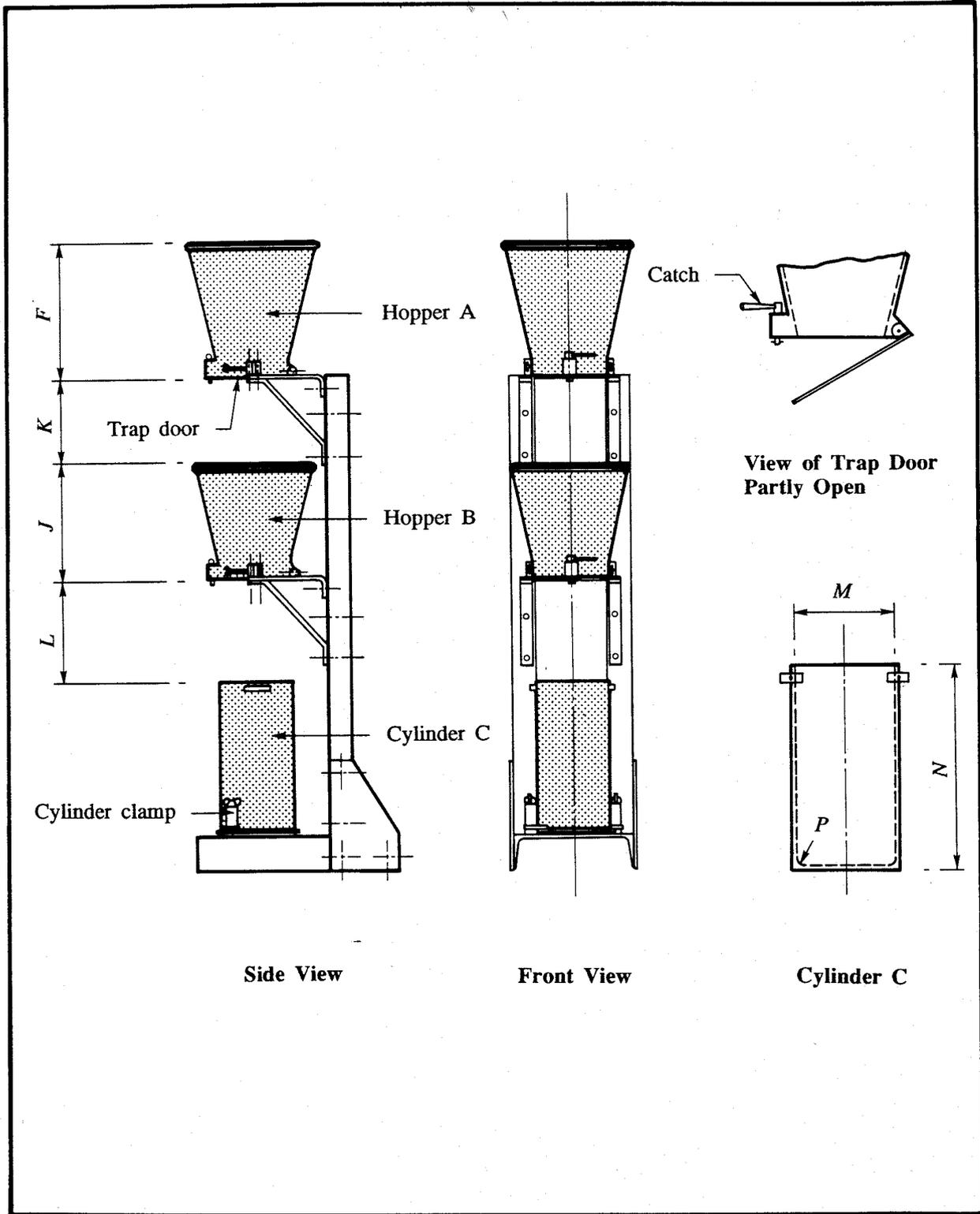
Figure 3 - Compacting Factor Apparatus
