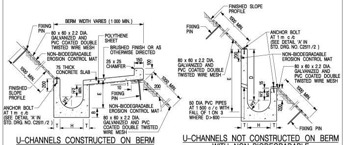
U-CHANNELS CONSTRUCTED ON BERM WITH NON-BIODEGRADABLE EROSION CONTROL MAT <u>J-CHANNELS NOT CONSTRUCTED ON BERM</u>
