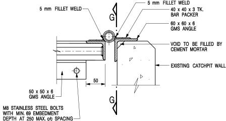
SECTIONAL ELEVATION (DETAIL 'H')
