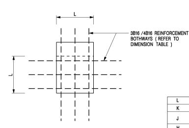
VIEW NORMAL TO SOIL NAIL HEAD FOR SPRAYED CONCRETE SLOPE SURFACE SCALE 1:20
