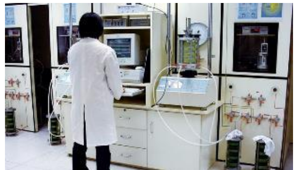
Triaxial Test of soil samples in PWL
