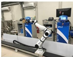
Automated Steel Rebar Testing System
