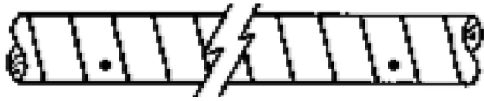
Distance between two ( ● ) marks approximate 26~92 ribs and 450~1200mm c/c (SGP2) Natsteel Ltd.
