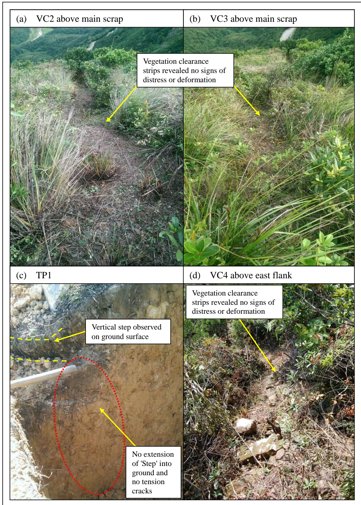
Figure 5.4 View of GI Works including Vegetation Clearance Strips and Trial Pit (Photograph taken on 6 and 13 October 2016)
