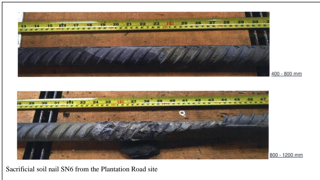
Figure 4.12 Example of Surface Conditions of Hot-dip Galvanized Soil Nails with Grout Sleeve in Exhumation Exercise in 2013
