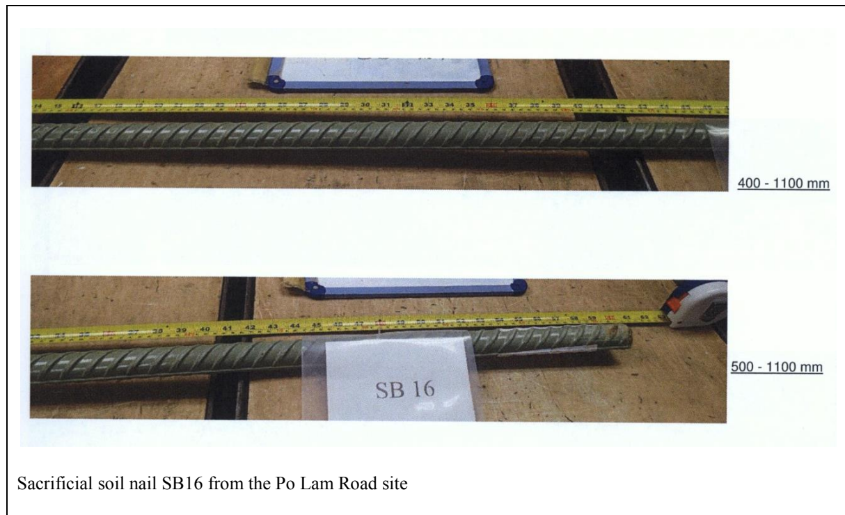
Figure 4.8 Example of Sacrificial Epoxy Coated Soil Nails with No Signs of Damage of Protective Coating in Exhumation Exercise in 2013
