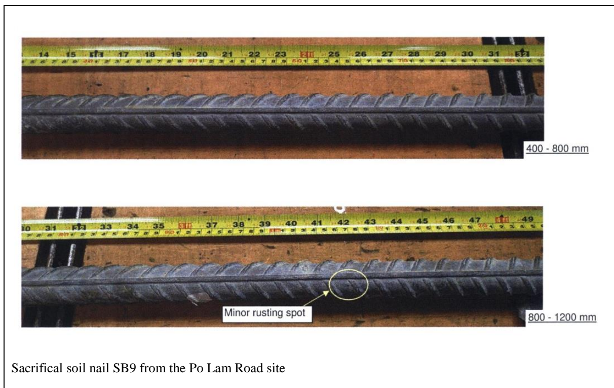
Figure 4.7 Example of Sacrificial Hot-dip Galvanized Soil Nails with No Significant Signs of Surface Corrosion in Exhumation Exercise in 2013
