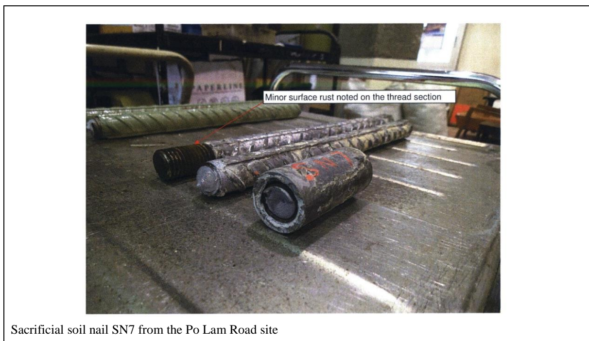
Figure 4.13 Example of Surface Conditions of Couplers in Exhumation Exercise in 2013
