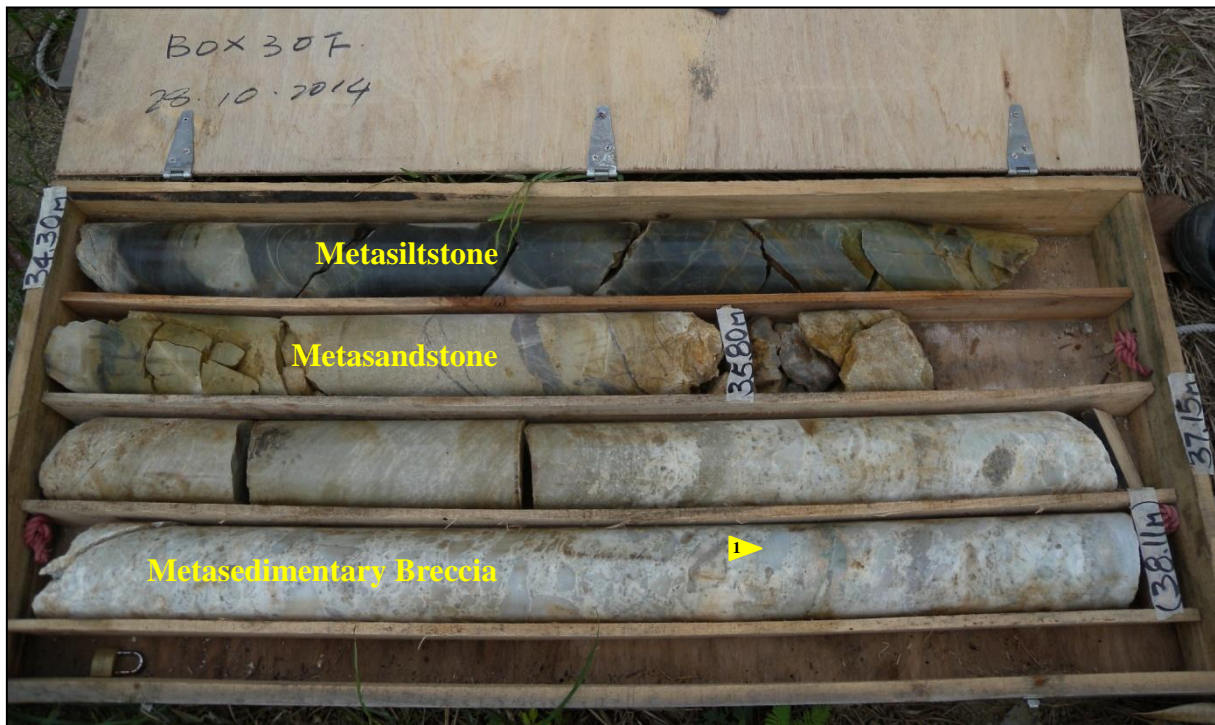
Figure 4.4 Normally-graded Metasedimentary Breccia-Metasandstone-Metasiltstone Sequence with an Apparent Thickness of c. 5 m (from 38.45 m to 33.40 m). (The metasedimentary breccia comprises many intensely altered clasts (arrow 1) with garnet mineralisation. The strata were previously assigned to Carboniferous Lok Ma Chau Formation by Langford et al (1989) and Frost (1992)) (Tin Shui Wai Area 115, Drillhole No. DH14, Box 3)
