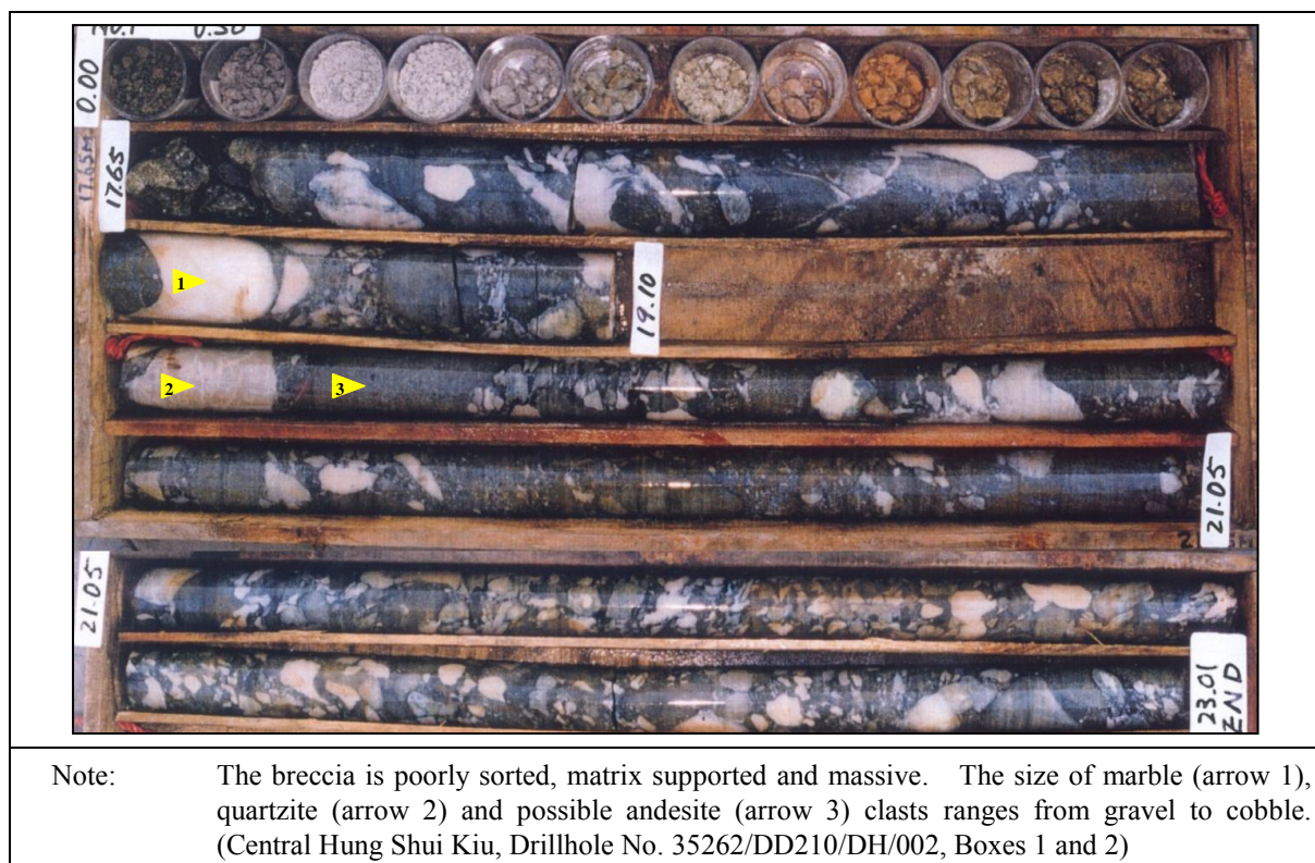
Figure A13 Altered, Calcareous, Tuffaceous Breccia with Many Marble Clasts
