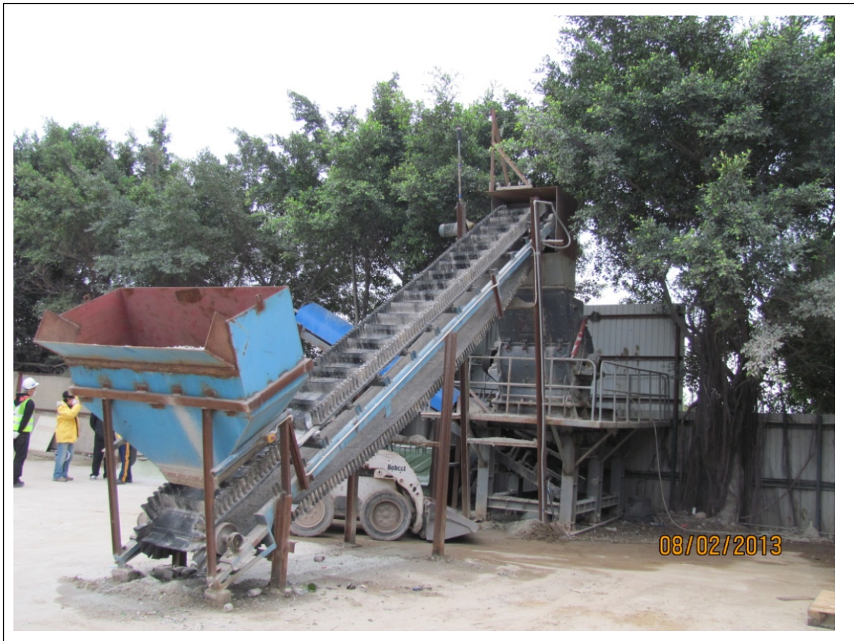
Figure 4.2 Production of Glass Cullet by Crushing of Waste Glass
