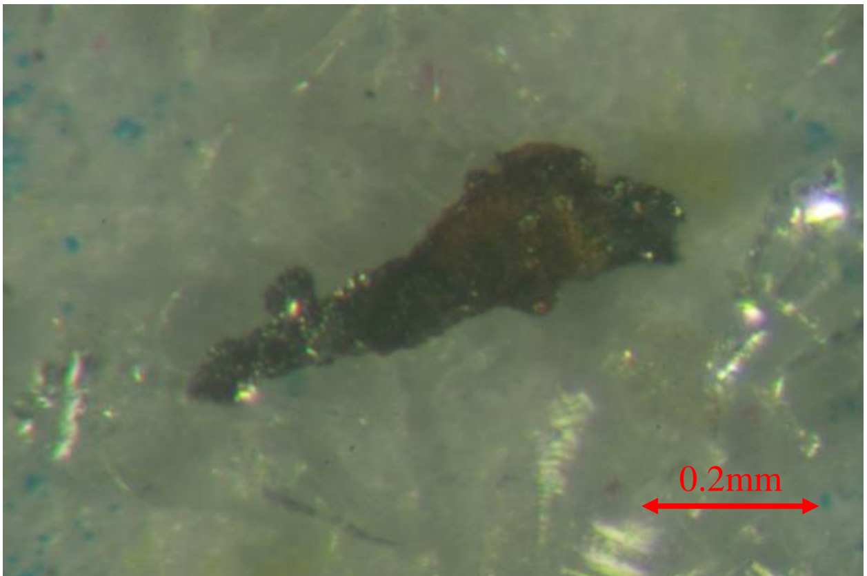
Plate 4: A Rust Flake with Metallic Luster Found in Sample CLSOR0800035A63
