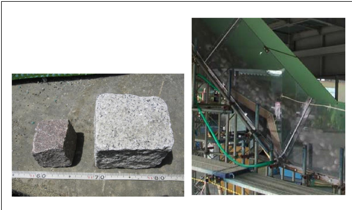
Figure 2.3 Left: Rock Blocks Used in the Flume Tests by Yang et al (2011); Right: Flume Test Involving Ballistic Flight of Rock Blocks
