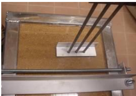
(e) Installation of TDR/WCR Probes Using the Model Probe
