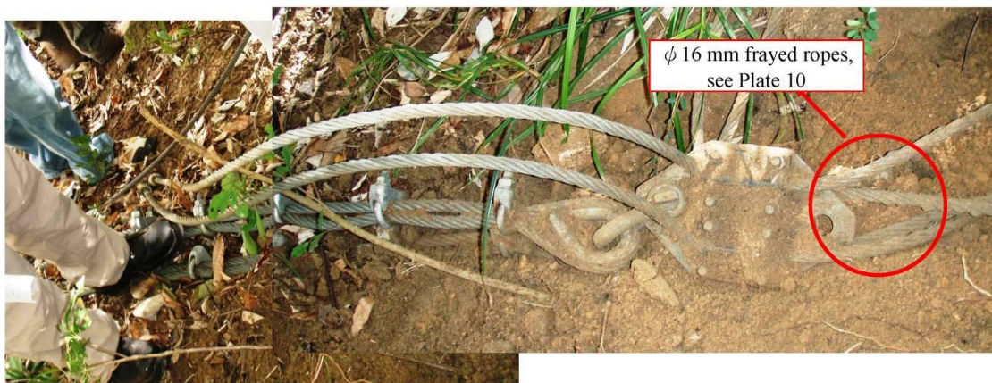
Plate 11 – Ropes Might Have Been Extended Slightly at the Monobloc Brake Connected to the Lateral Anchor
