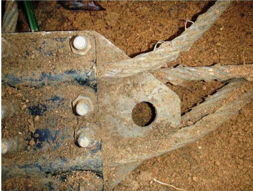
Plate 10 – Frayed Ropes Connected to the Braking System of the Lateral Anchor
