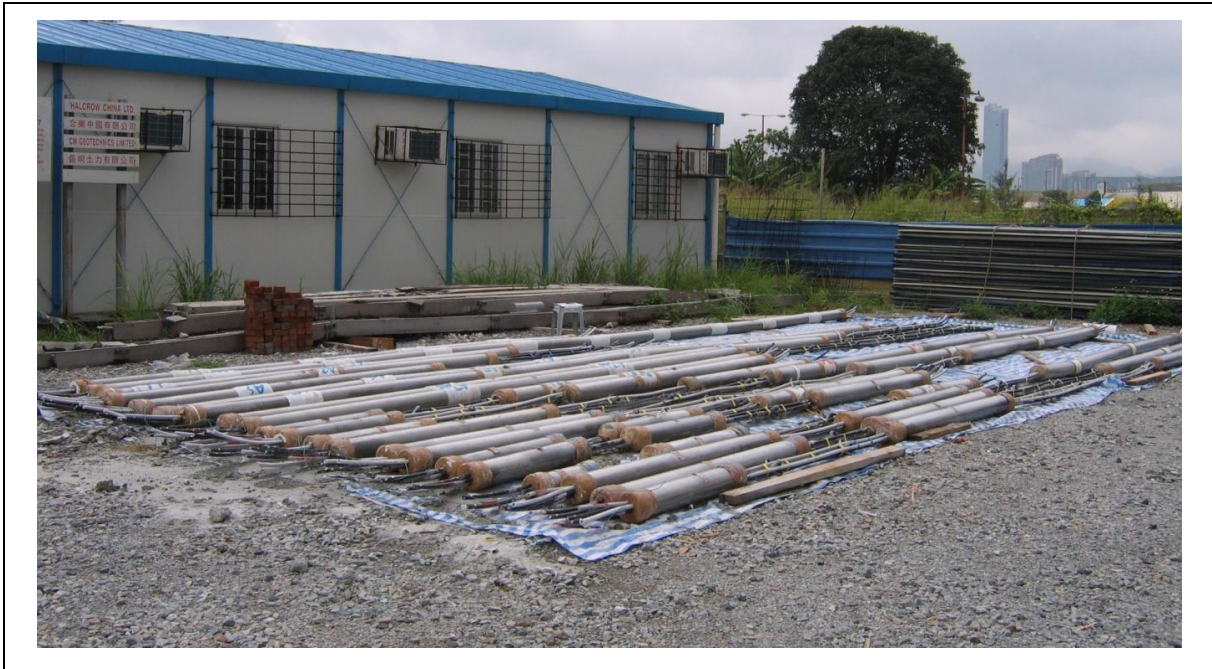
Figure 3.1 Prefabricated Soil Nails with Built-in Grout Defects
