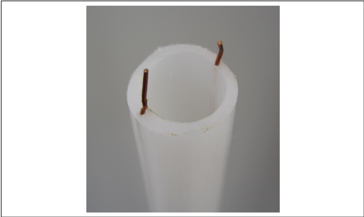
Figure 3.3 Grout Pipes with Embedded Copper Wires
