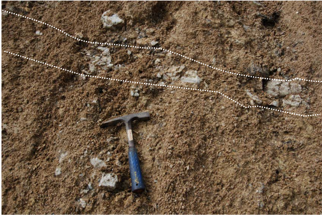
Plate 25 - Close-up View of the Quartz Vein Exposed in the Lower Portion of the Source Area (Photograph taken on 10 June 2008)
