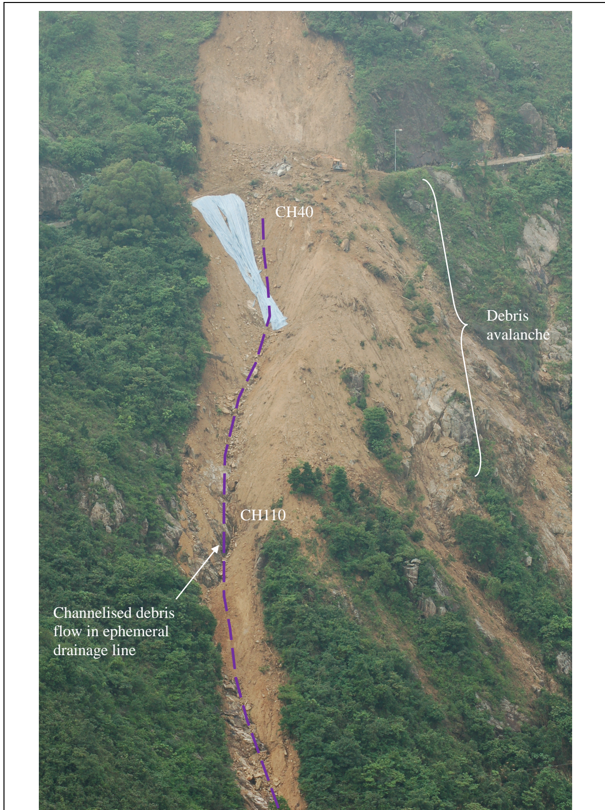
Plate 28 - Oblique Aerial View of the Upper Channelised Debris Flow Path (Photograph taken on 16 June 2008)
