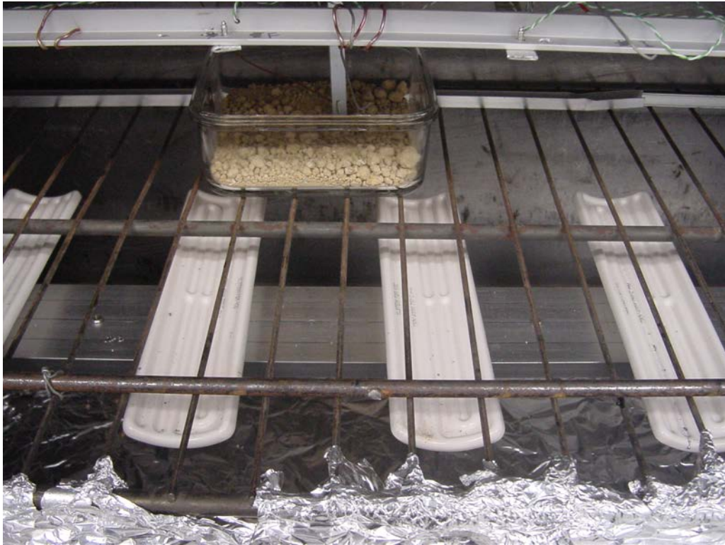
Plate 1 – Concave-shape Infrared Heating Panels Used in this Study
