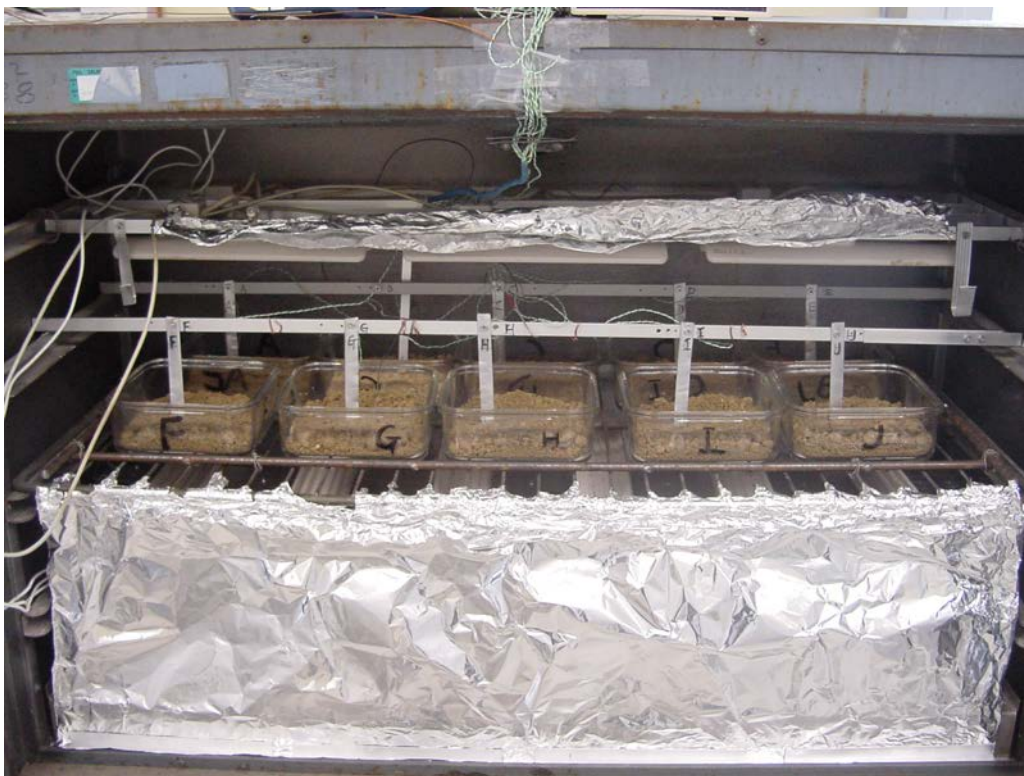
Plate 4 – Layout of Glass Containers with the Provision of Temperature Sensors
