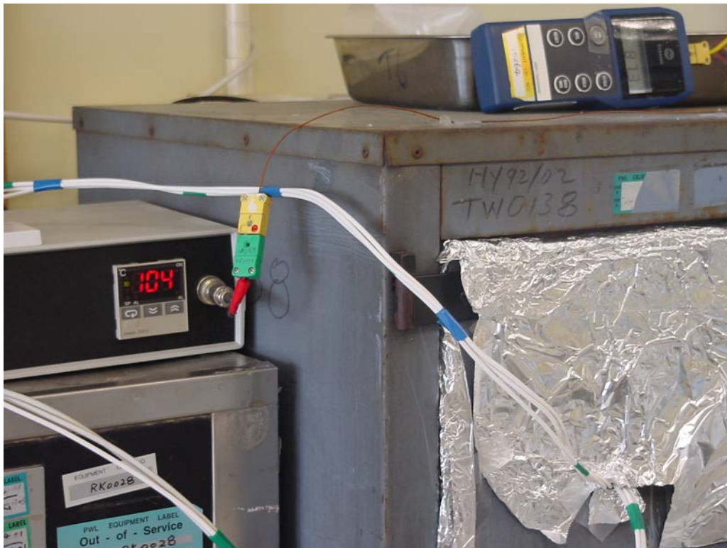
Plate 7 – Power Control Device to Regulate the Power Supply to Infrared Heating Panels
