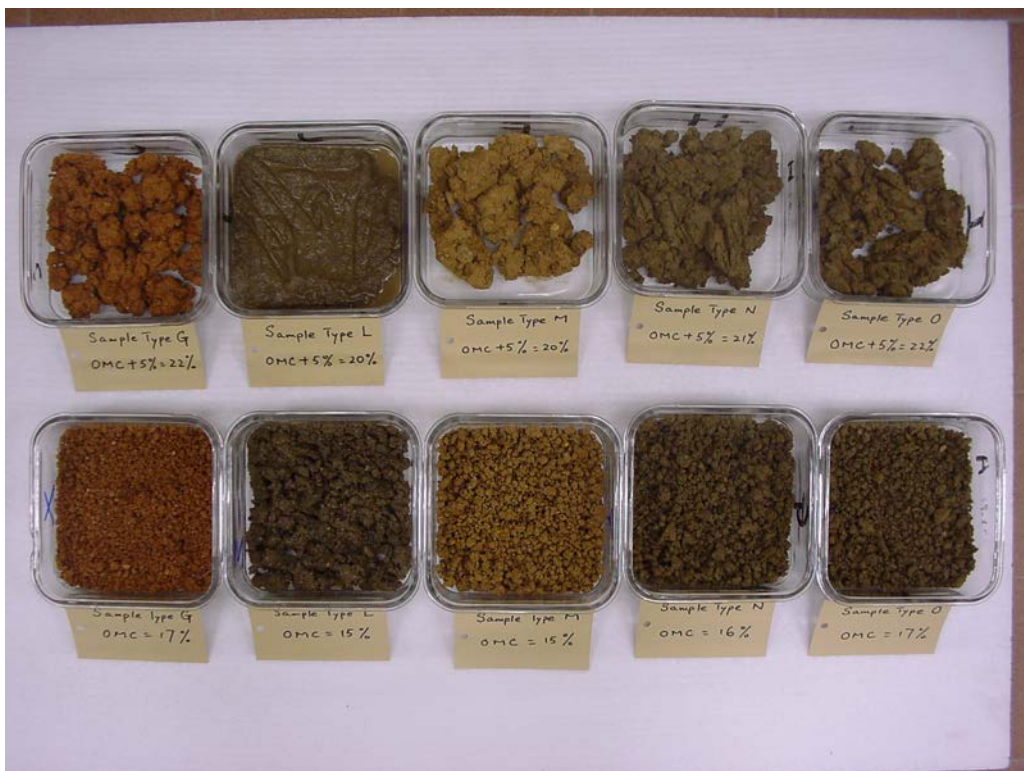
Plate 8 – Conditions of Selected Samples with Moisture Content at OMC and OMC + 5%
