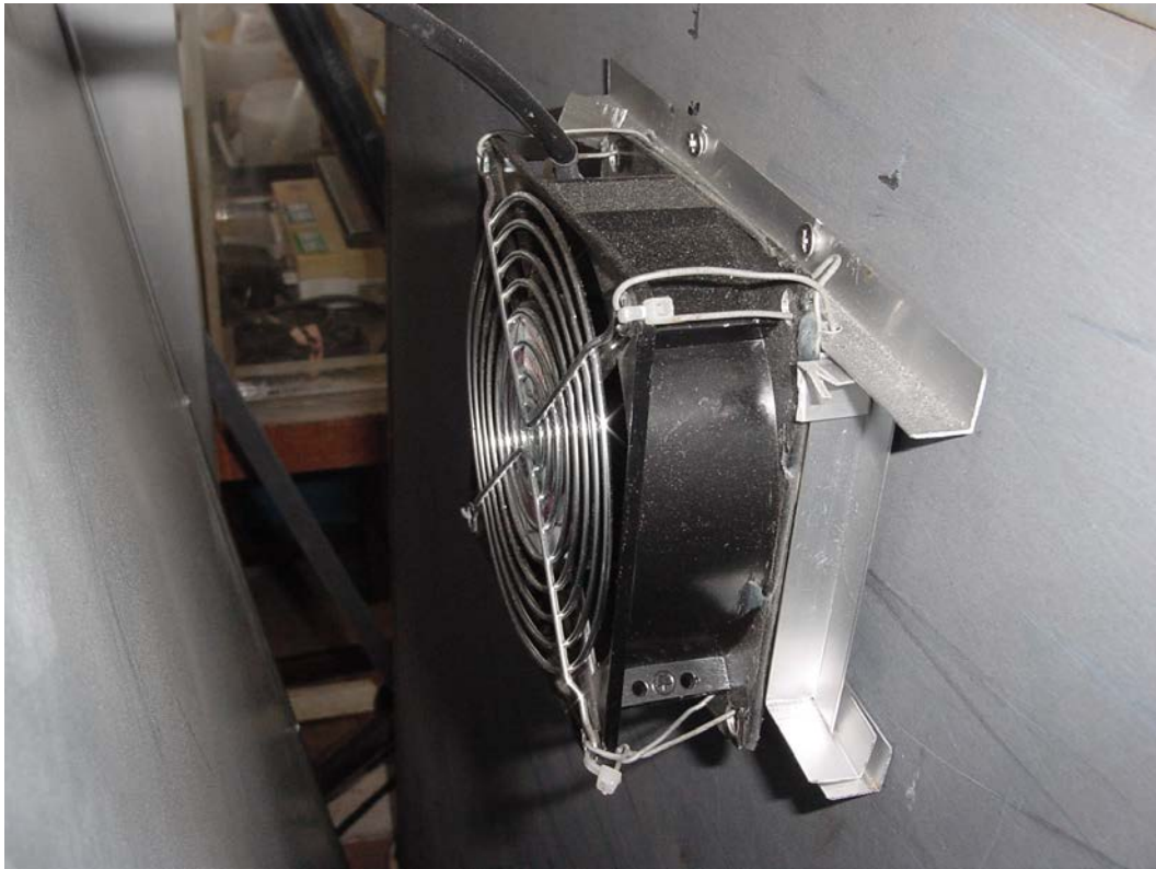
Plate 5 – Provision of an External Fan at the Rear Side of the Oven
