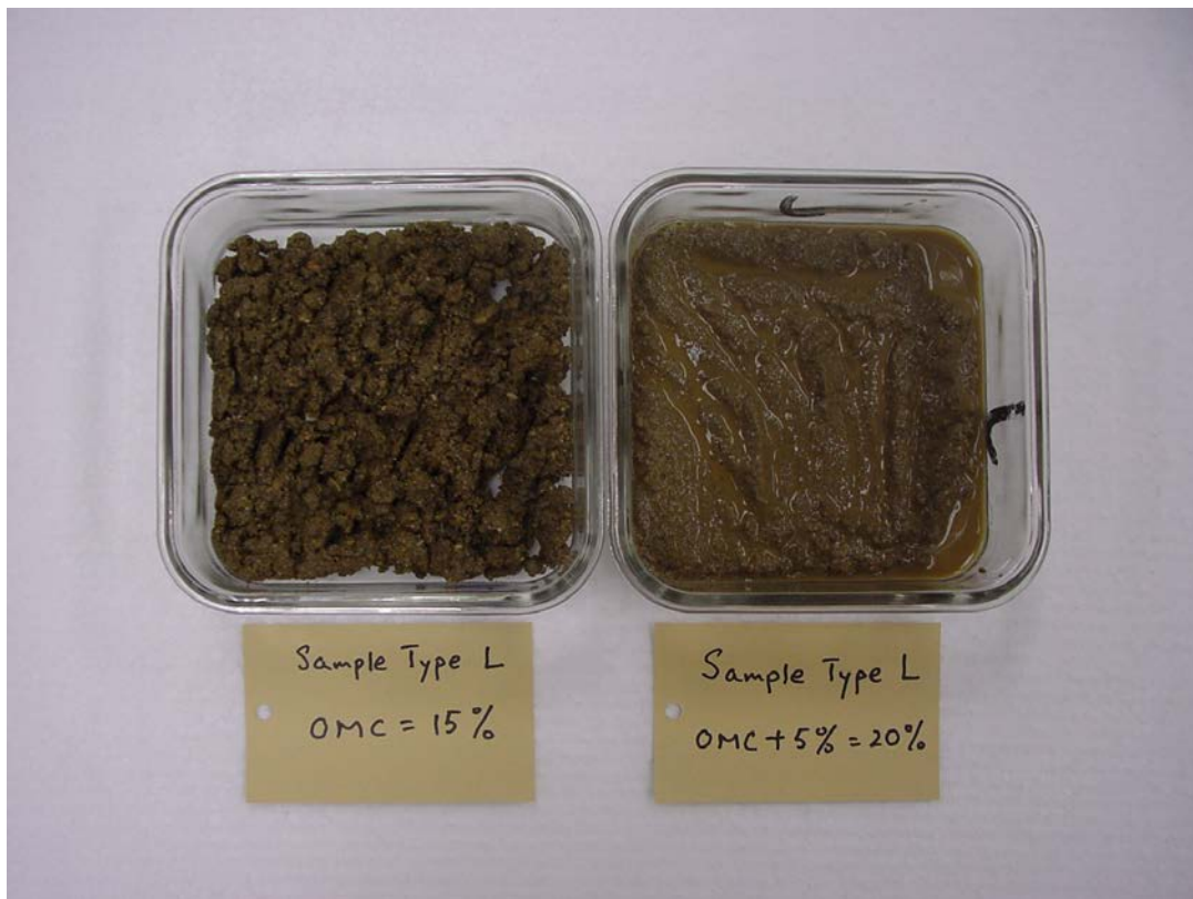
Plate 9 – Sample Very Wet at Moisture Content of OMC + 5%
