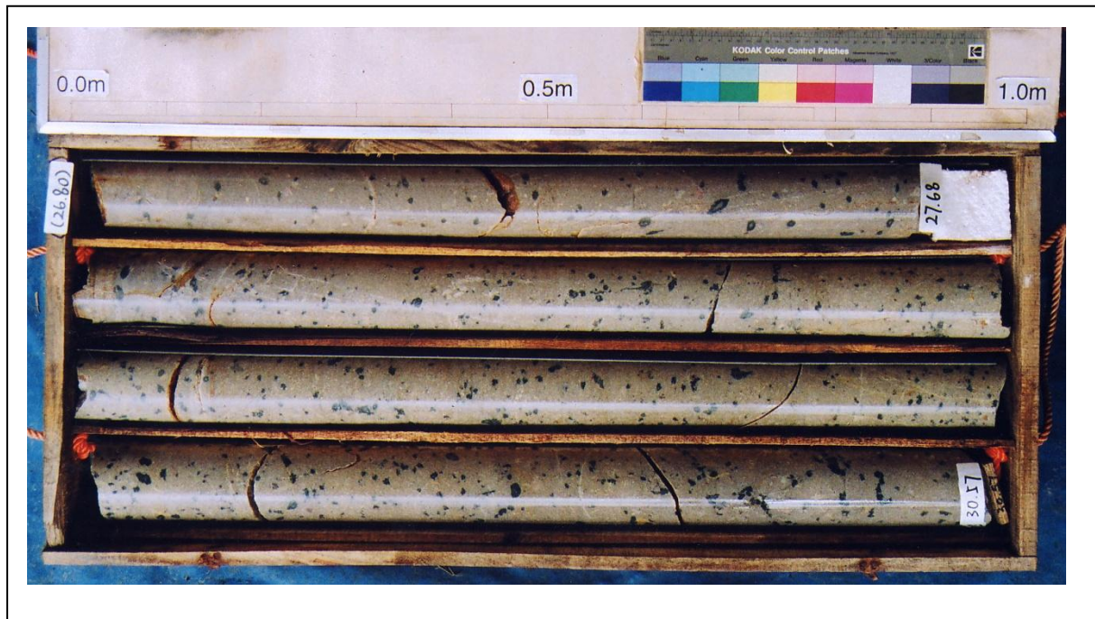
Figure 4.1 Corebox Photograph of Contact Metamorphosed Tuffaceous Rock (Hornfels), Western Hong Kong Island
