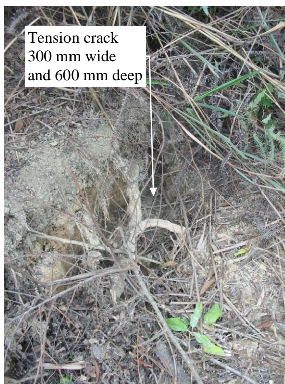
Plate 11 - Tension Crack on Area above Slope No. 6NE-B/C44 (Photograph taken on 19 November 2007)
