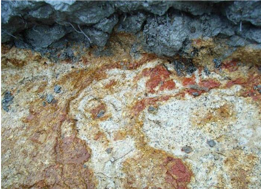
Plate 22 - Kaolin Infill Observed in Slope Surface Strip No. SS1 (Photograph taken on 26 May 2009)
