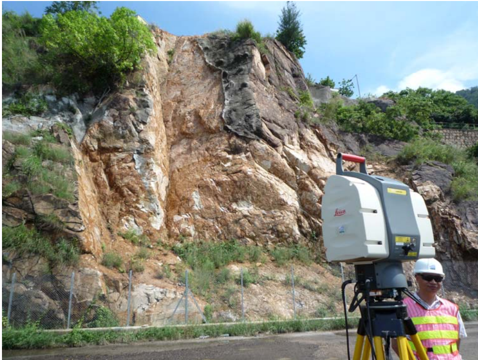
Plate 16 - Remote Laser Scanning Method for Rock Joint Mapping (Photograph taken on 6 July 2009)
