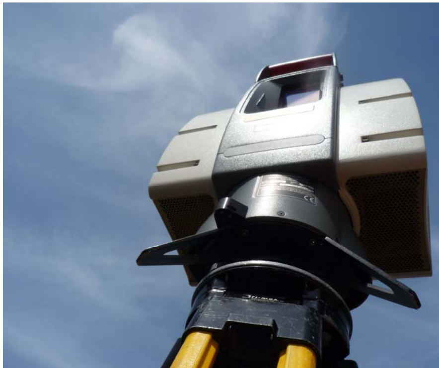
Plate 17 - High-Definition Surveying Laser Scanner Developed by Leica Geosystems (Photograph taken on 6 July 2009)
