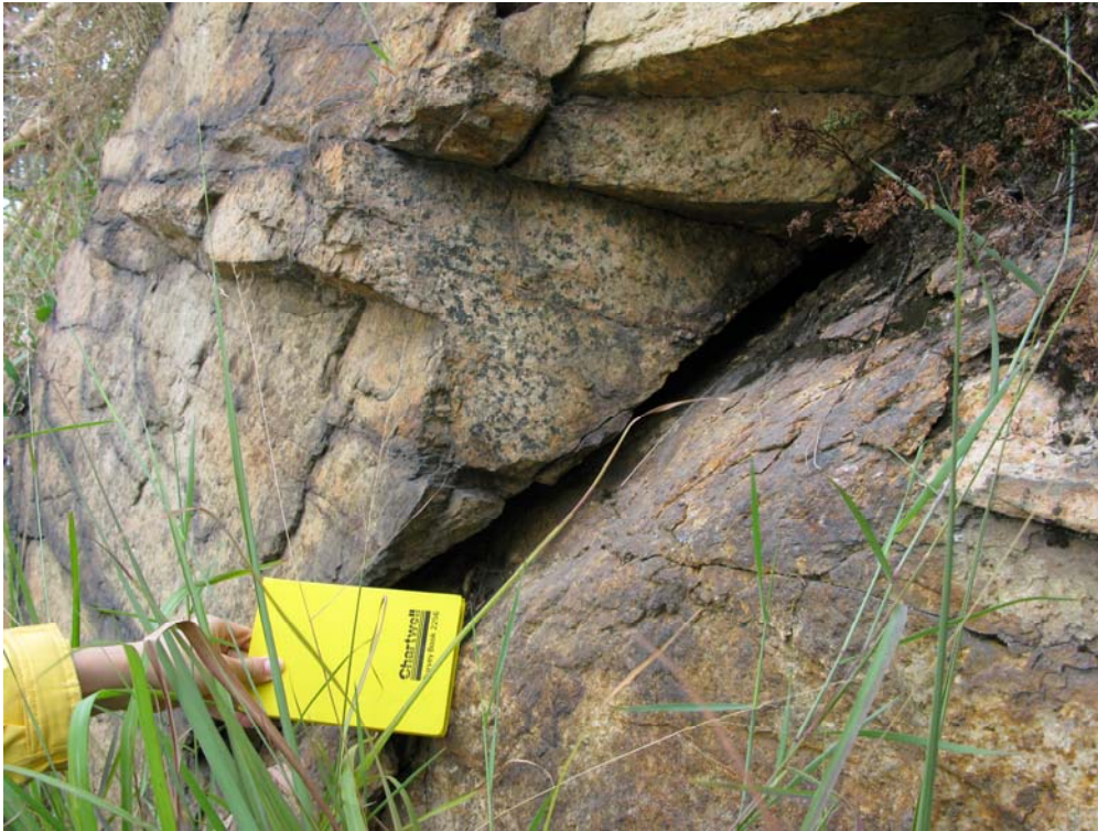
Plate 12 - Opening-up of Rock Joint Observed Close to the Scar (Photograph taken by 20 October 2009)
