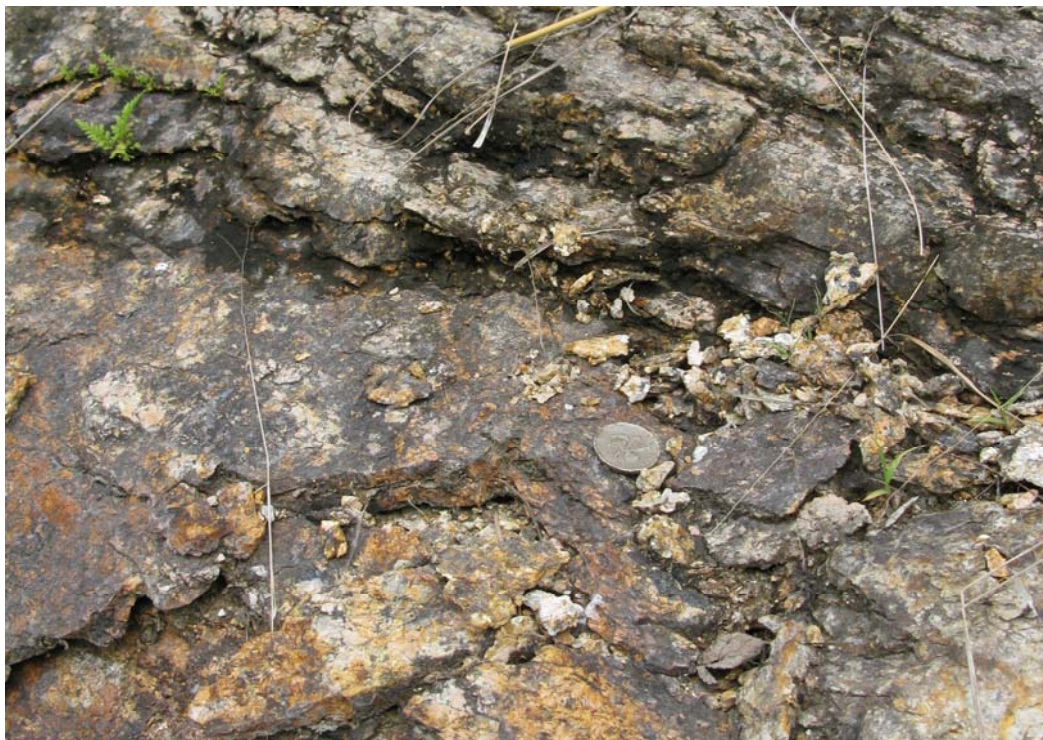
Plate 8 - Close View of the Basal Slip Surface (Photograph taken on 20 October 2009)
