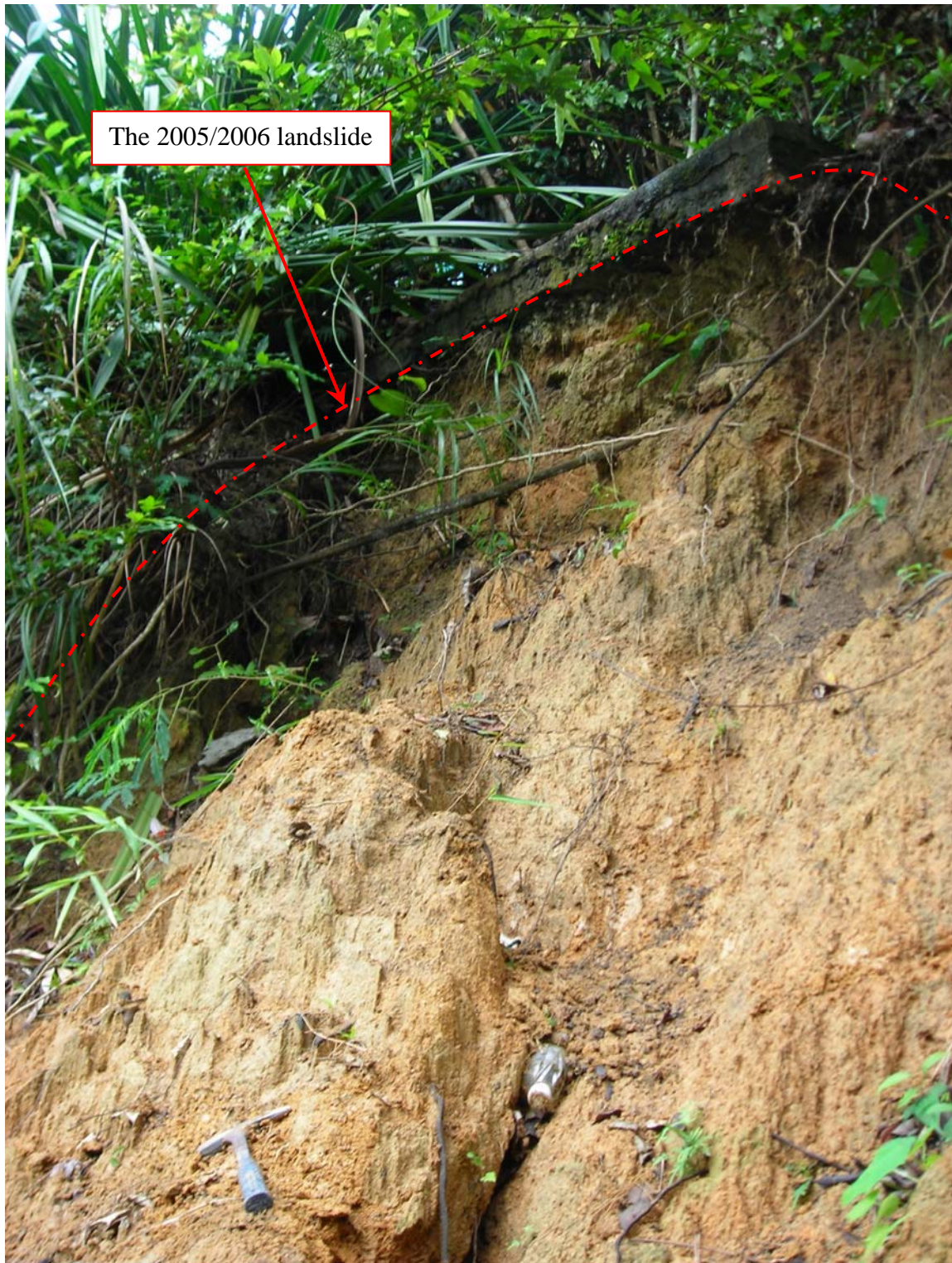
Plate 10 - General View of the 2005/2006 Landslide below Wall No. 11SE-C/R7 (Photograph taken on 3 October 2007)
