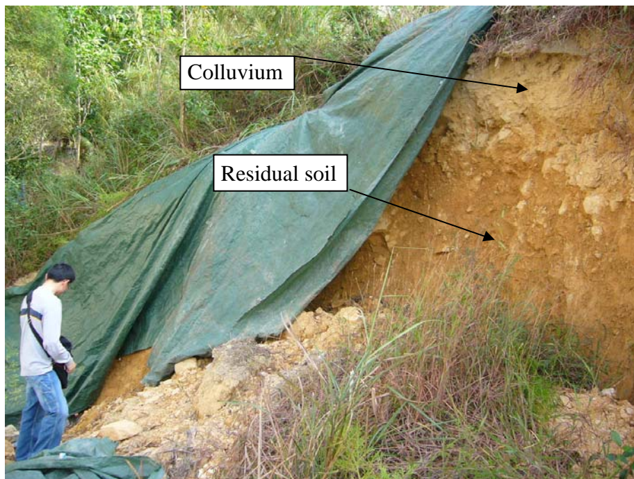
Plate 6 - Soil Materials Exposed on the Back Scarp of the Landslide Site (Photograph taken by MGSL on 14 November 2005)
