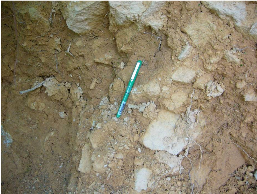
Plate 9 - Completely Decomposed Tuff Exposed on the Landslide Debris (Photograph taken by MGSL on 14 November 2005)
