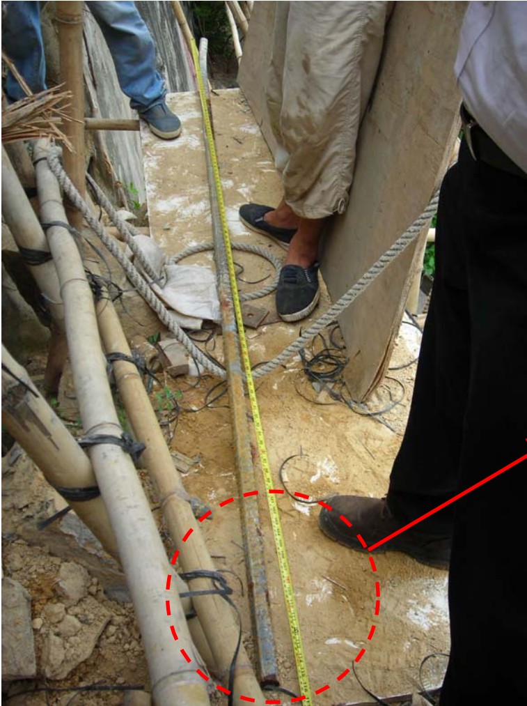
Plate 13 – Exhumed Soil Nail Reinforcing Bar (Photograph taken on 4 September 2006)
