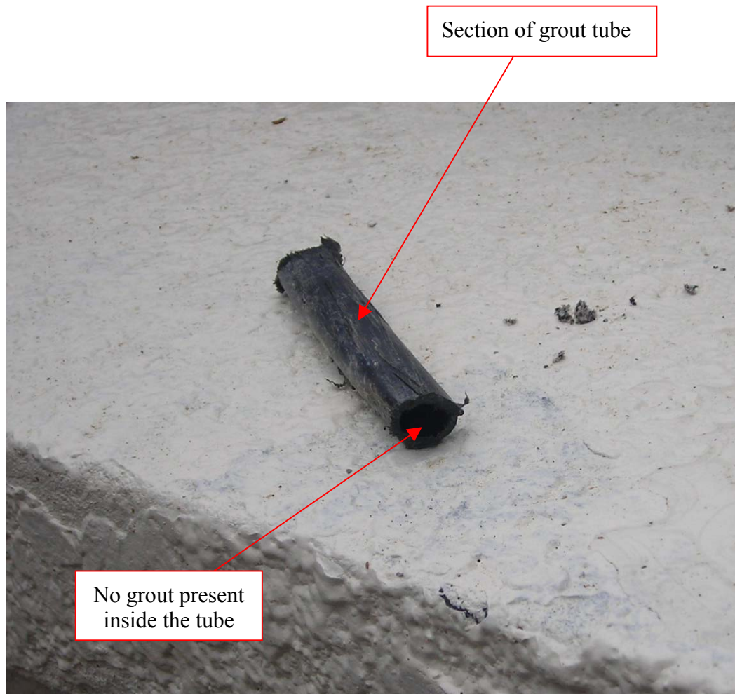
Plate 14 – Section of Grout Tube Recovered from Soil Nail Drillhole (Photograph taken on 4 September 2006)
