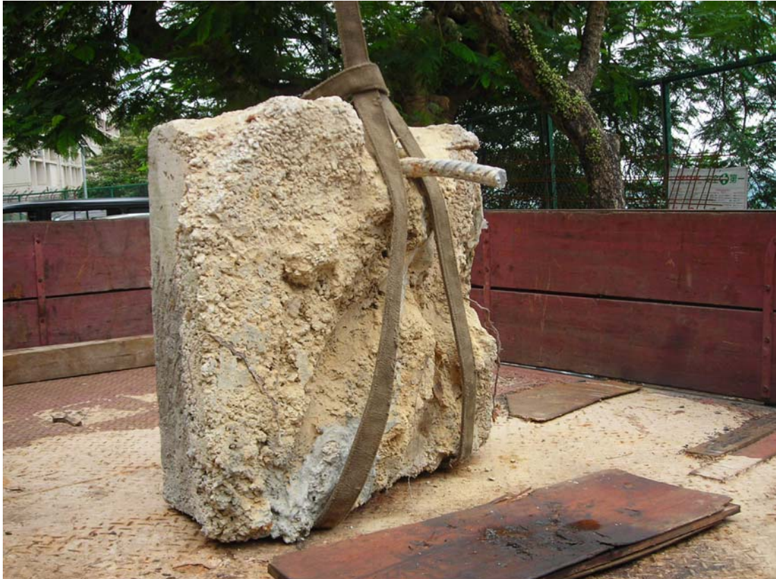
Plate 11 – Soil Nail Head Following Detachment from Reinforcing Bar (Photograph taken on 4 September 2006)
