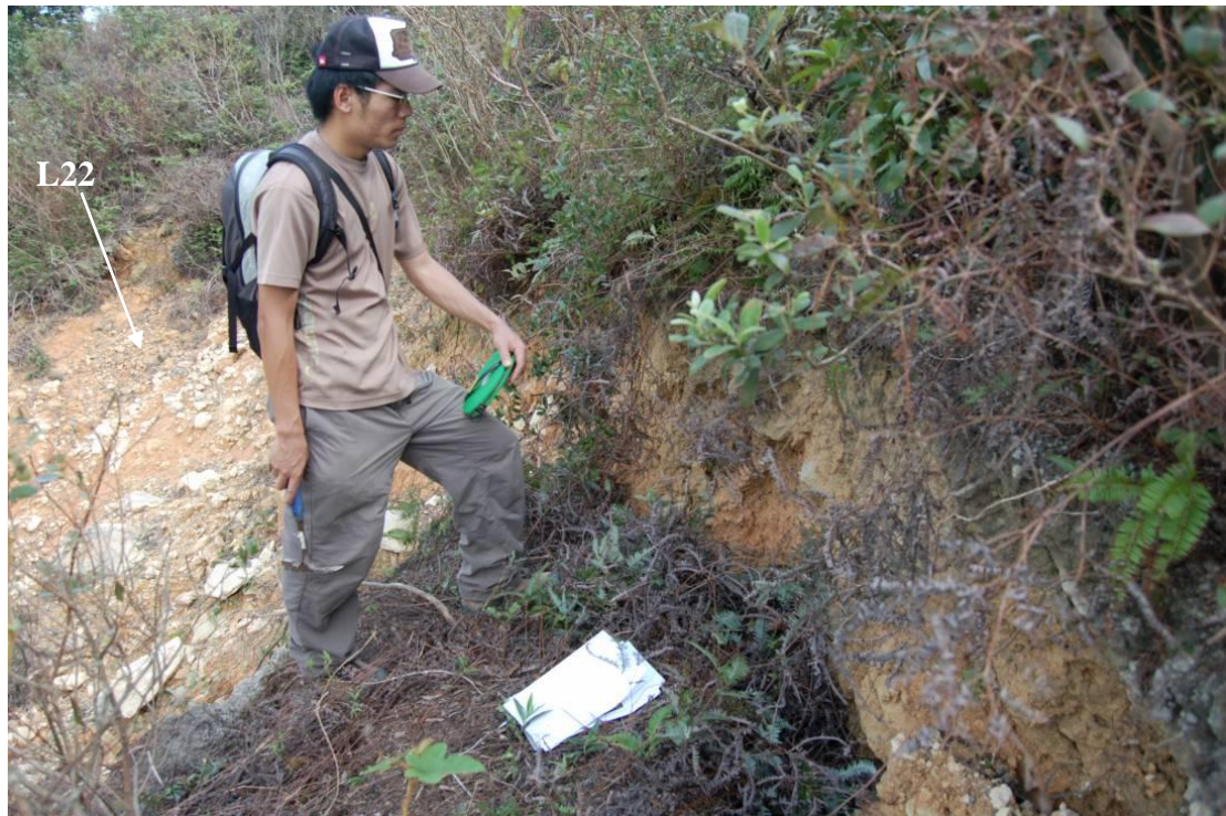
Plate 11 - View of Tension Crack between Landslides Nos. L22 and L41 (Photograph taken on 10 October 2008)
