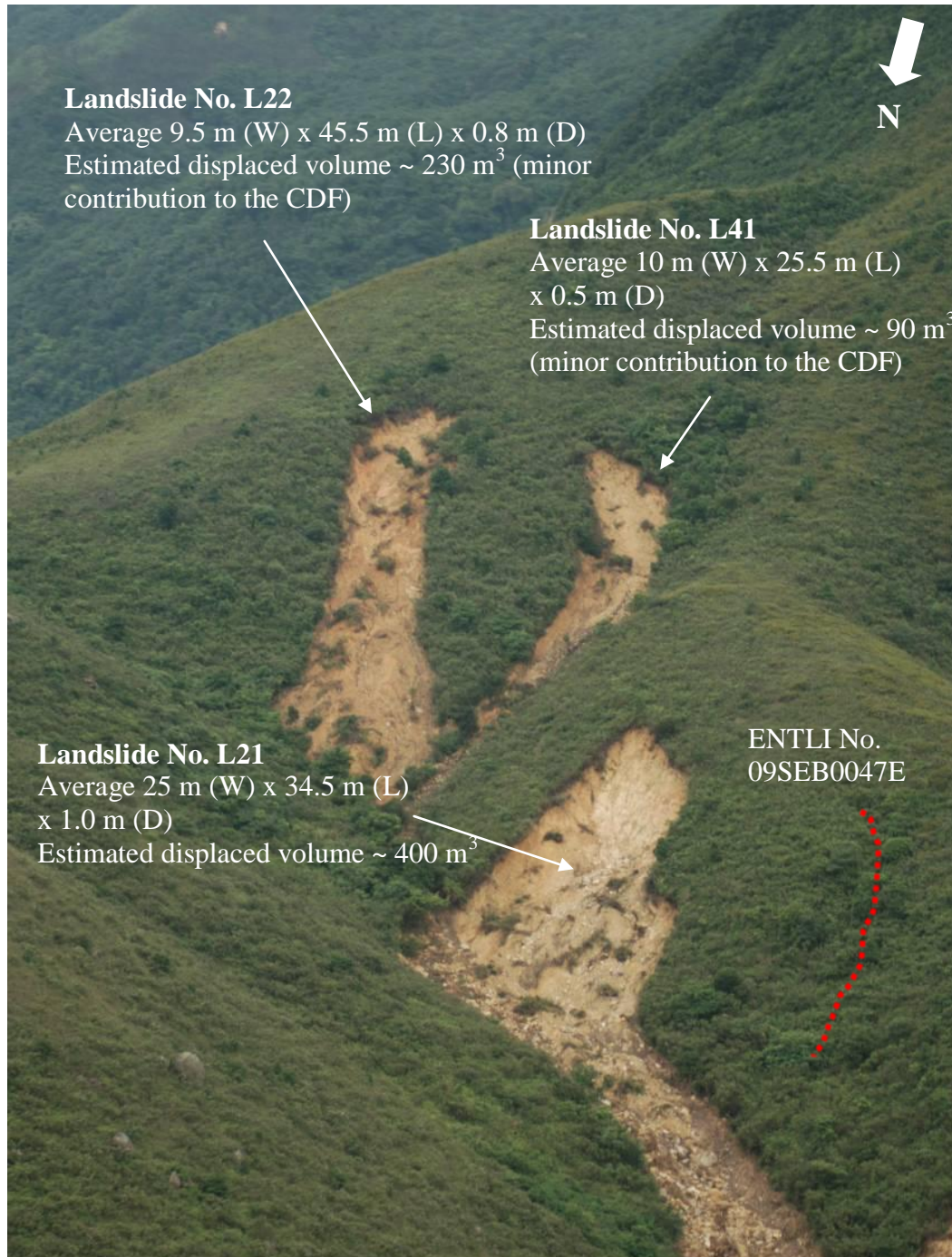
Plate 8 - Oblique Aerial View of Landslides Sources at Head of Catchment No. 15 (Photograph taken on 16 June 2008)
