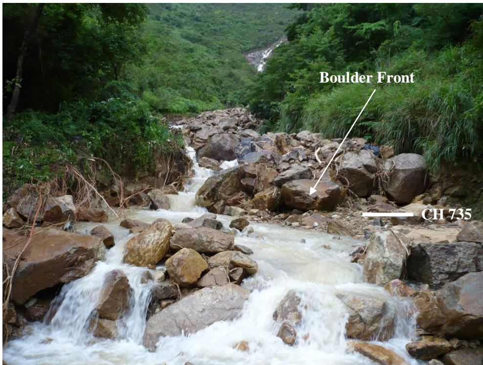
Plate 25 - About 300 m 3 of Matrix-Supported Bouldery Debris Observed at CH735, along the Northern Drainage Channel with a Gradient of 5° to 10° in Catchment No. 15 (Photograph taken at about 1 pm on 7 June 2008)
