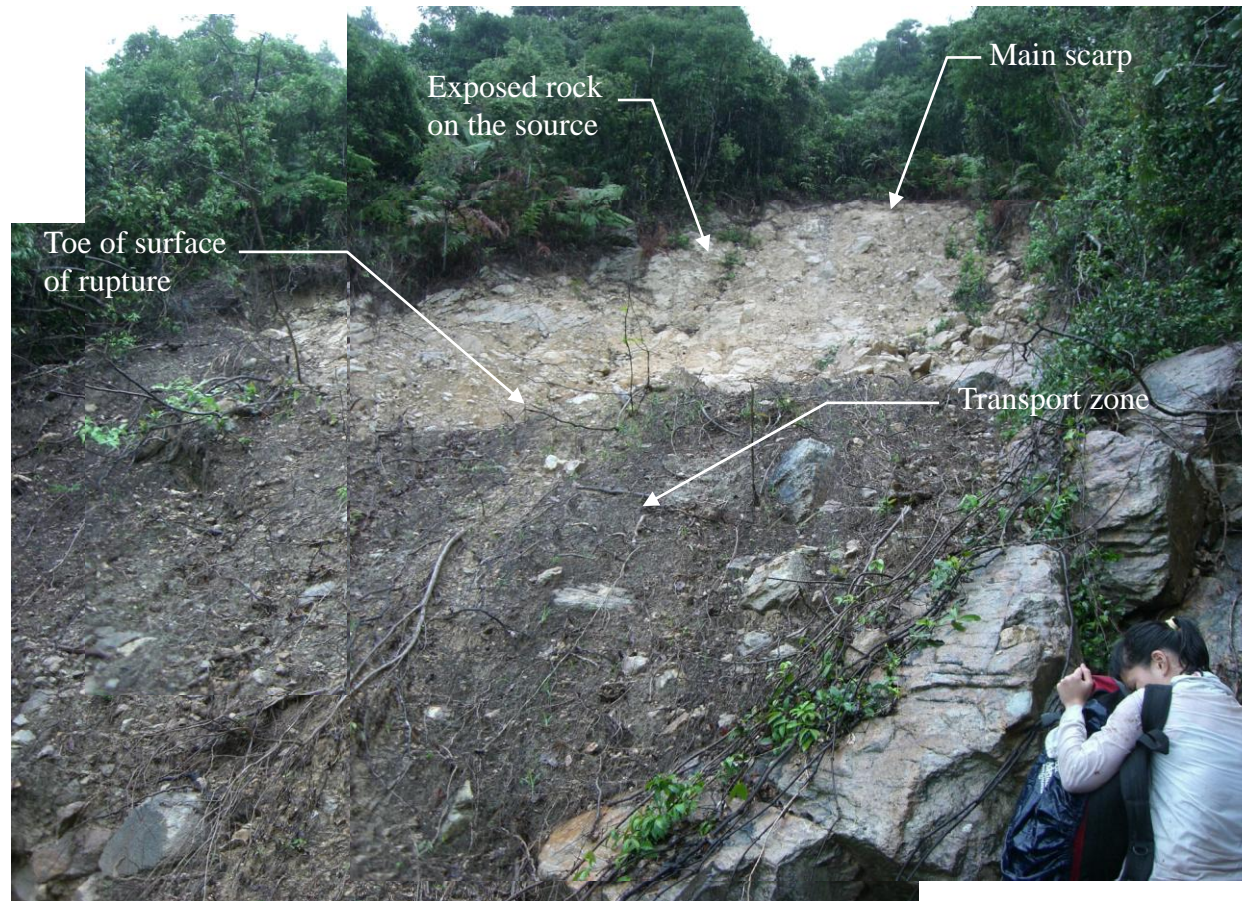
Plate B7 - View of Landslide Source Area of Landslide No. L4 in Catchment No. 21 (Photograph taken on 11 August 2008)
