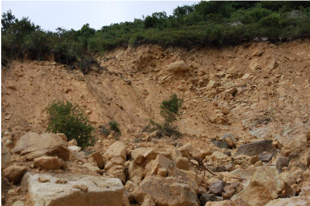
Plate 29 – Talluvium Exposed in Backscarp of Source of Landslide No. L25 in Catchment No. 30 (Photograph taken on 14 June 2008)
