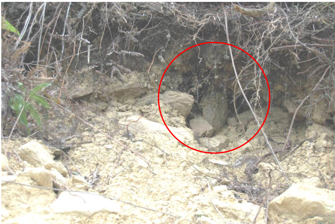
Plate 9 - Voids in Colluvium at Landslide No. L3 in Catchment No. 24 (Photograph taken on 15 June 2008)
