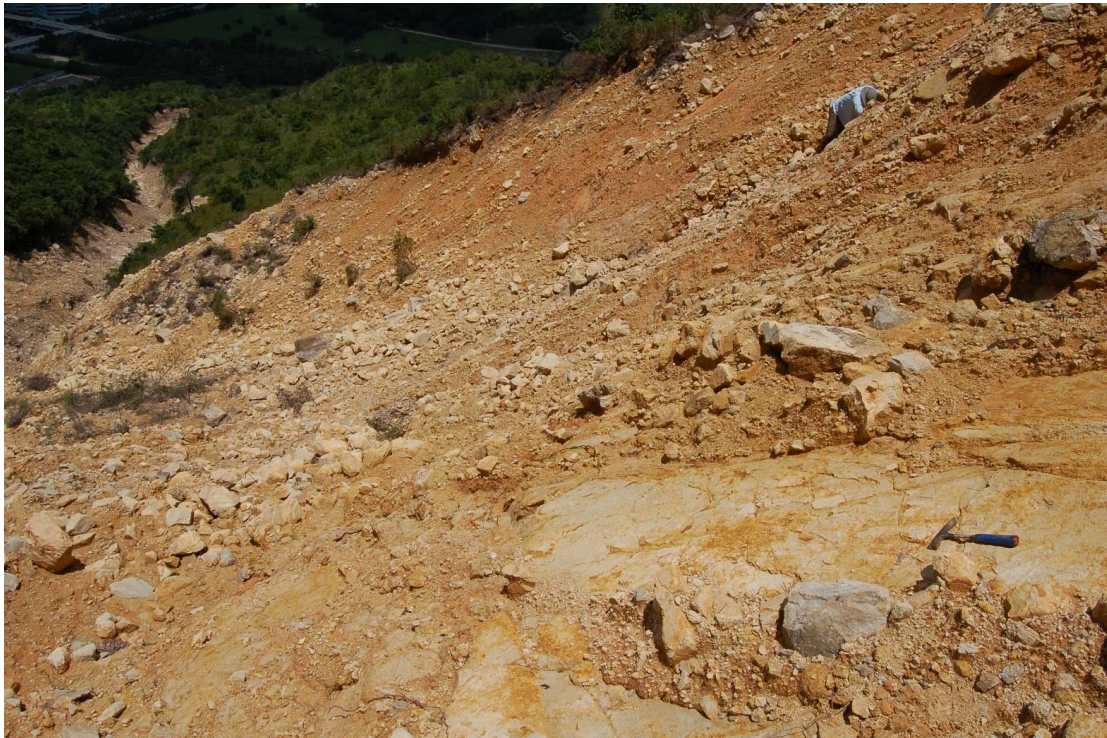
Plate 31 – Planar Joint Moderately Decomposed Tuff in Base of Landslide Scar at Landslide No. L25 in Catchment No. 30 (Photograph taken on 21 July 2008)
