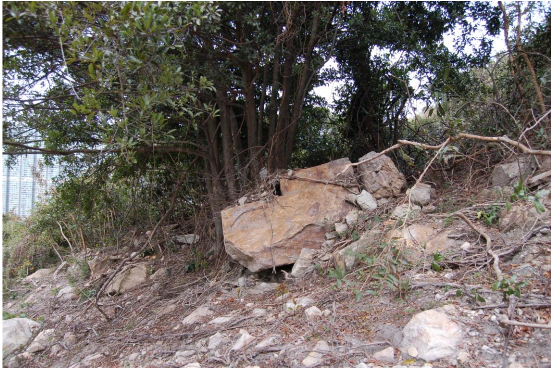
Plate 12 – Debris Levees with Large Boulders of up to 2 m Diameter along the Side of the Debris Trail at about CH255 in Catchment No. 24 (Photograph taken on 7 June 2008)
