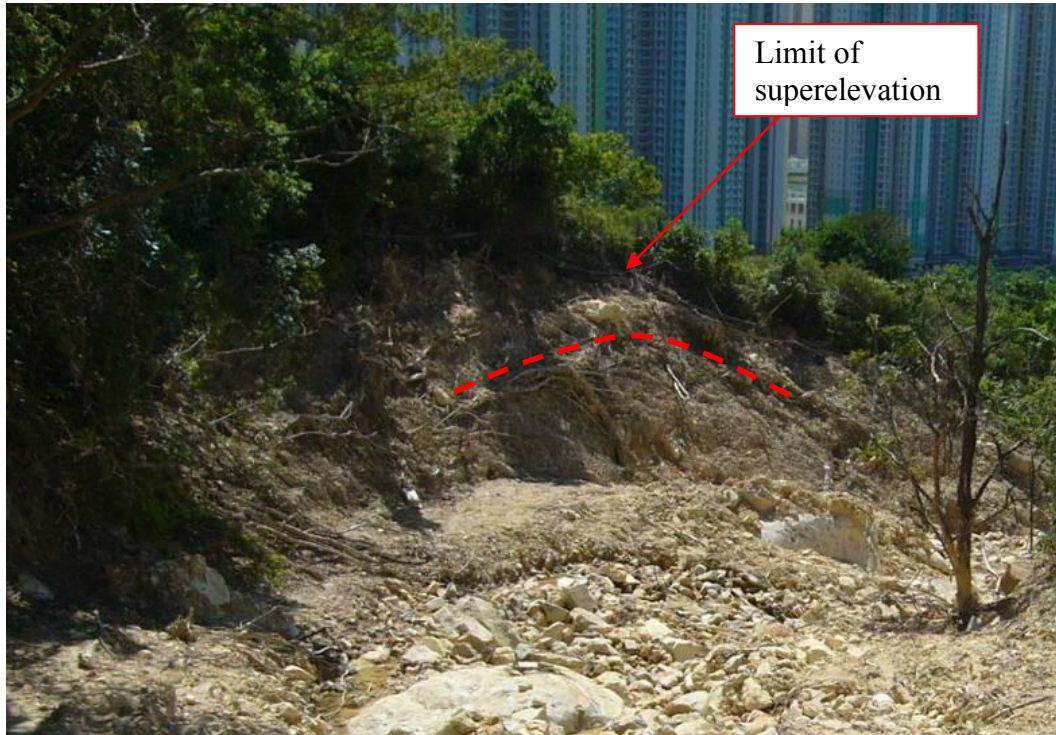
Plate 35 – View of Western Flank of Drainage Line at CH413 Showing Superelevated Debris (Photograph taken on 25 July 2008)
