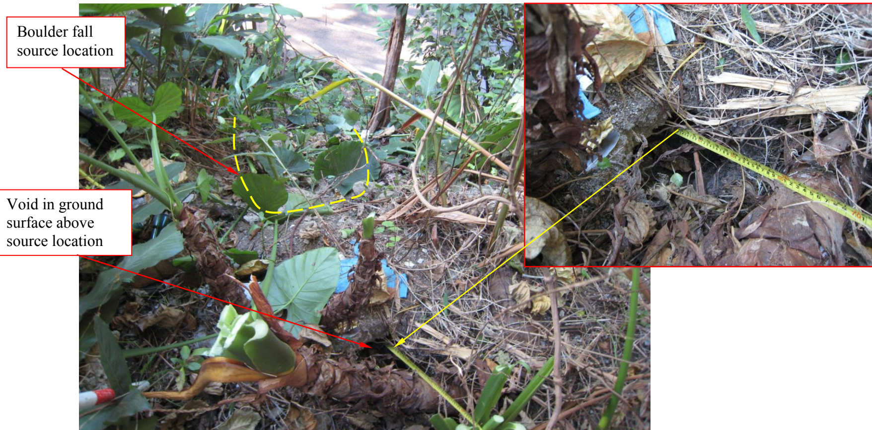
Plate 25 - Void in Ground Surface above 27 May 2007 Boulder Fall Source Location (Photograph taken on 25 October 2007)
