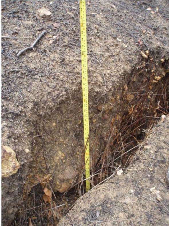
Plate 6 - Close-up of the Main Tension Crack at the North-facing Hillside (Photograph taken on 23 April 2007)
