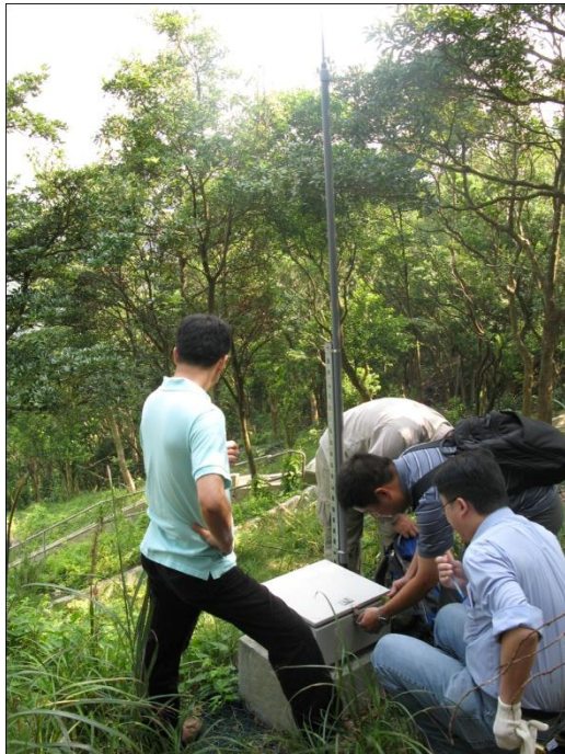
(a) Sensor node with extended antenna to improve data transmission range
