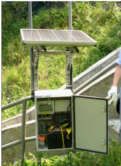
(c) Solar panel recharging the battery in the base station. Two antennae are installed for LAN and WAN
