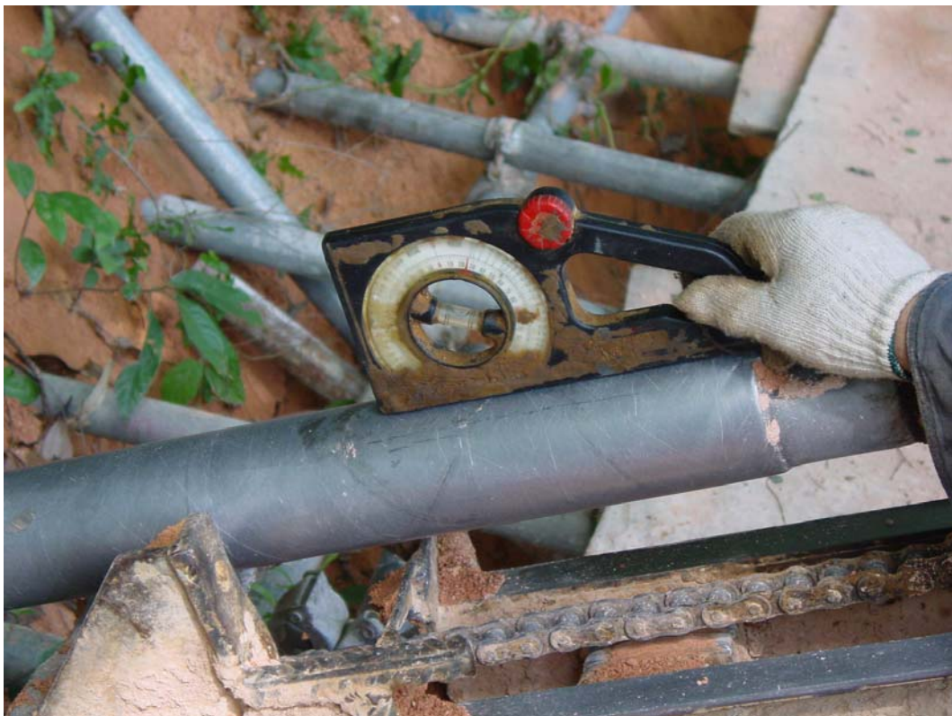
Plate 2 - Common Practice of Setting the Inclination of the Drilling Rig using a Protractor
