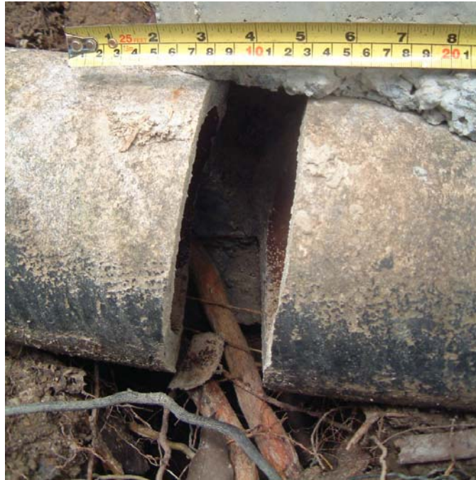
Plate 11 – View of Tensile Fracture in Existing Asbestos Pipeline (Photograph taken by FSW on 12 September 2005)
