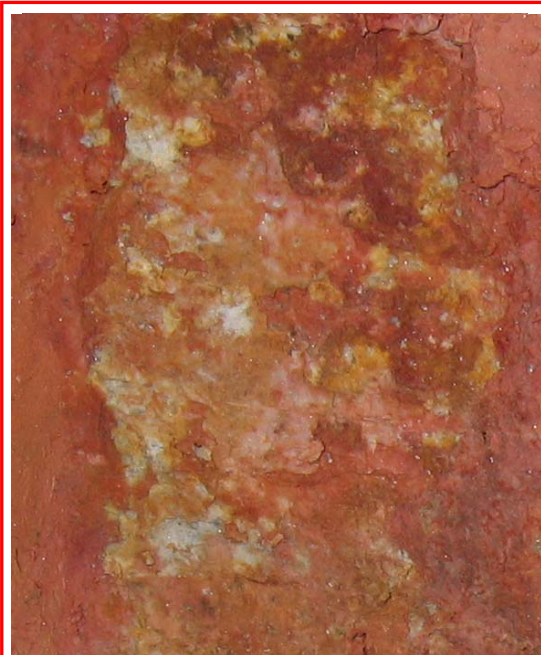
No voiding was observed within intact Grade V tuff
