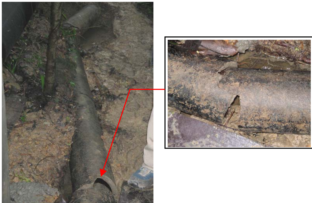
Plate 3 – Close-up View of the Severed Existing Asbestos Pipeline (Photograph taken by FSW on 24 August 2005)
