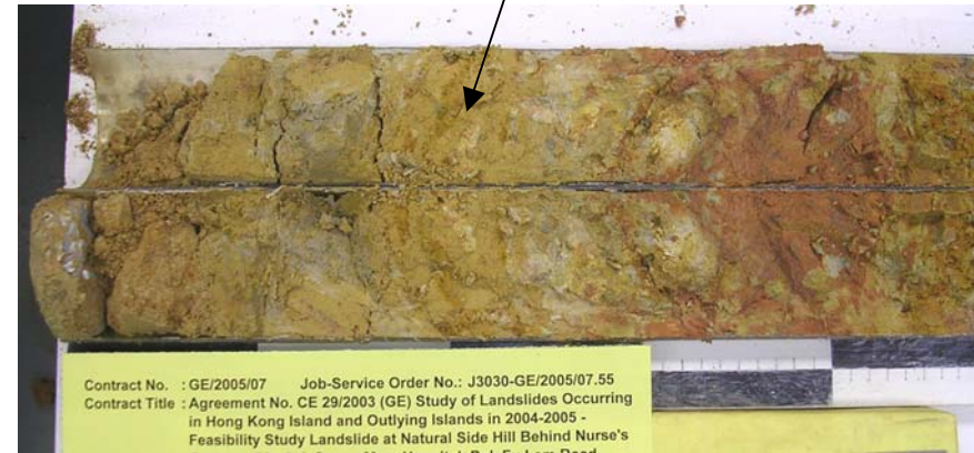
(b) Top of Mazier Sample from Drillhole BH2, Depth 2.6 m to 3.6 m
