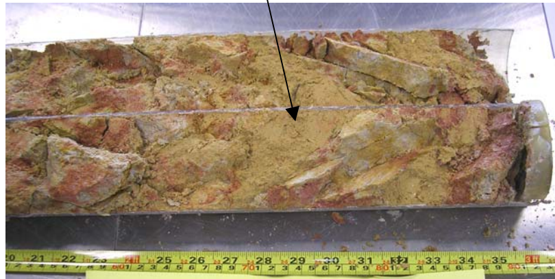
(a) Base of Mazier Sample from Drillhole BH2, Depth 1.5 m to 2.5 m
