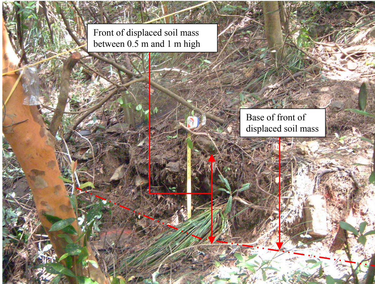
Plate 9 – View of Bulging in the Lower Southern Flank of the Landslide (Photograph taken by FSW on 28 September 2005)
