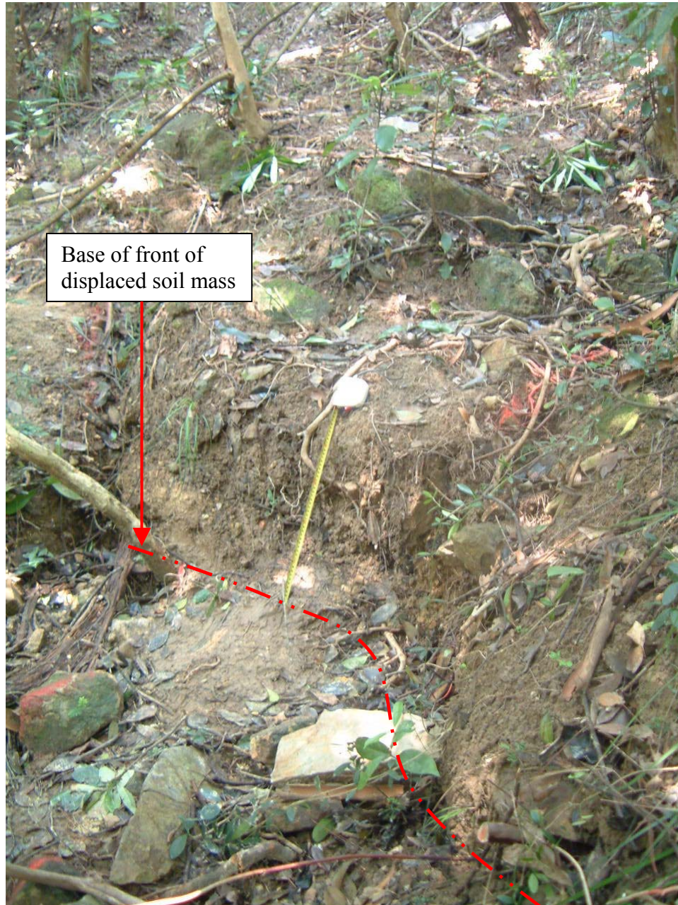
Plate 10 – View of Bulging at the Toe of the Landslide (Photograph taken by FSW on 28 September 2005)
