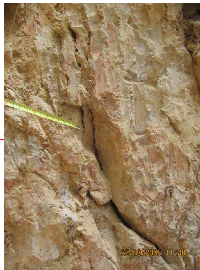
Plate 23 – View of Subsurface Cracking in Face B of Trial Trench TT2 (Photograph taken by FSW on 25 October 2005 and 19 November 2005)
