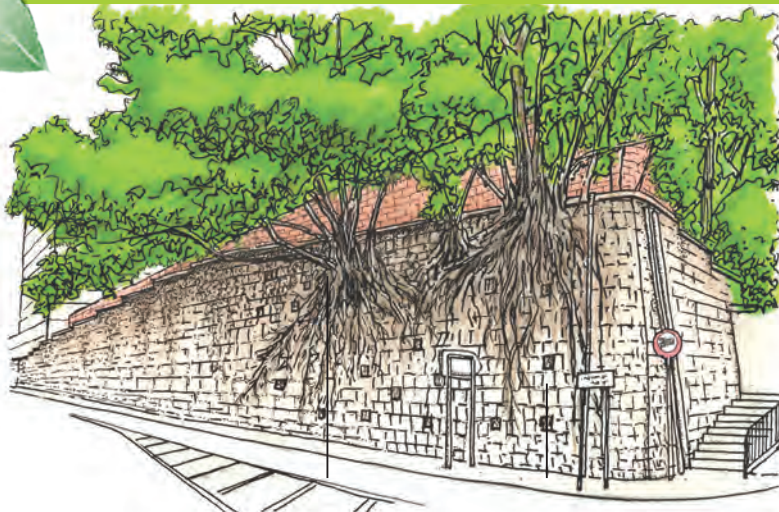
Use of soil nails to stabilise an existing masonry wall allows attractive “wall trees” to remain undisturbed
