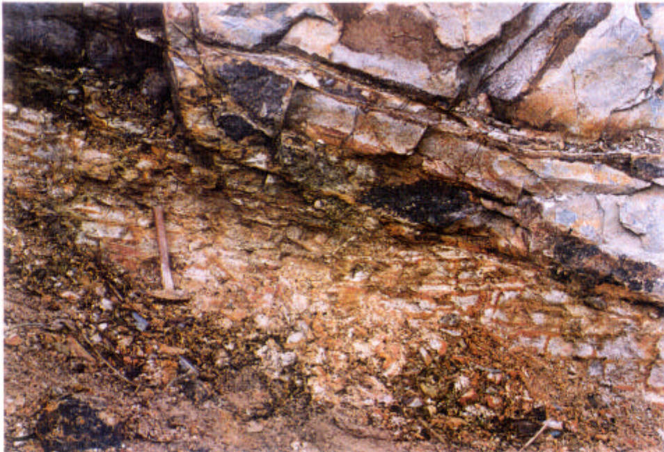
Plate 10 - Kaolinite-rich Altered Tuff at the Unfailed Portion of the Cut Slope to the East of the Landslide (Photograph Taken on 8 October 1995. See Figure 21 for Location)
