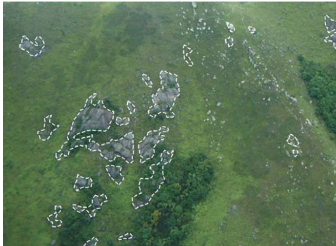
Oblique Aerial Photograph showing many small individual granite rock outcrops, Regolith Class Bg. Given the difficulty and time required to identify each outcrop, the Rg classification below can be used.
