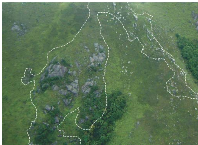
Oblique aerial photograph showing intermittent granite outcrops with typically less than 1.0 m of regolith cover in between, Regolith Class Rg.
