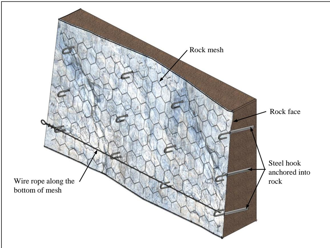
Figure 1 An example of fixing of rock mesh to the bottom of rock face
