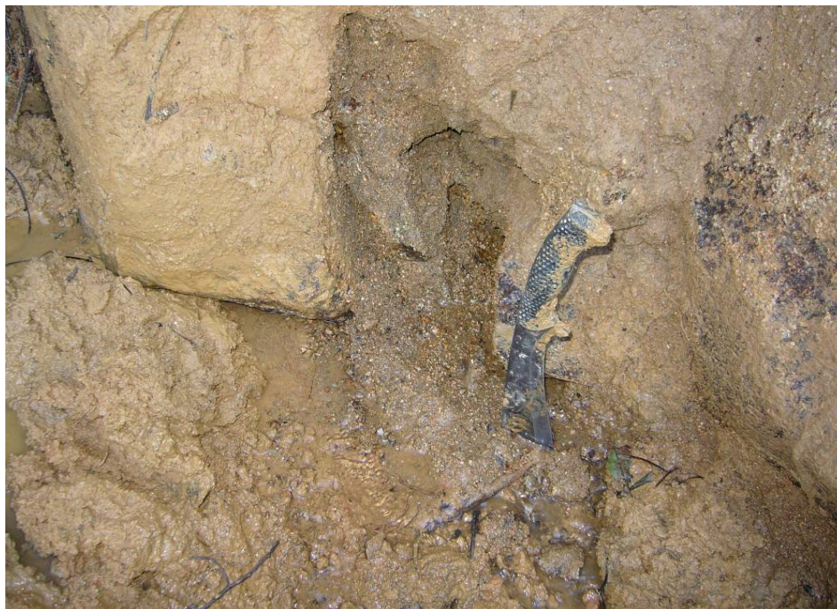
Plate 15 - Close-up View of Seepage at Centre of Main Scarp (Photograph taken on 29 August 2005)
