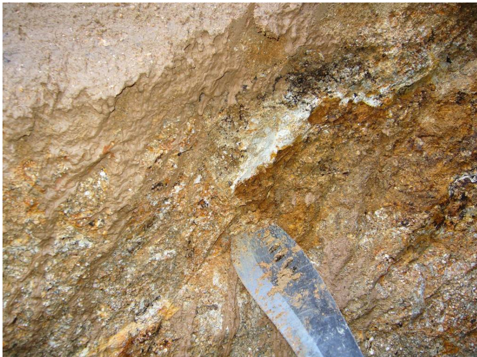
Plate 13 - Close-up View of Pocket of Kaolin Seam in Eastern Flank (Photograph taken on 29 August 2005)
