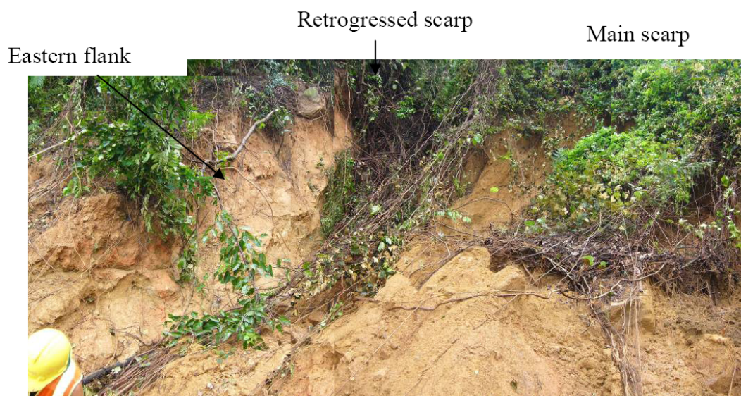
Plate 6 - General View of Source: Looking from Toe of Rupture towards Retrogressed Scarp (Photograph taken on 24 August 2005)
