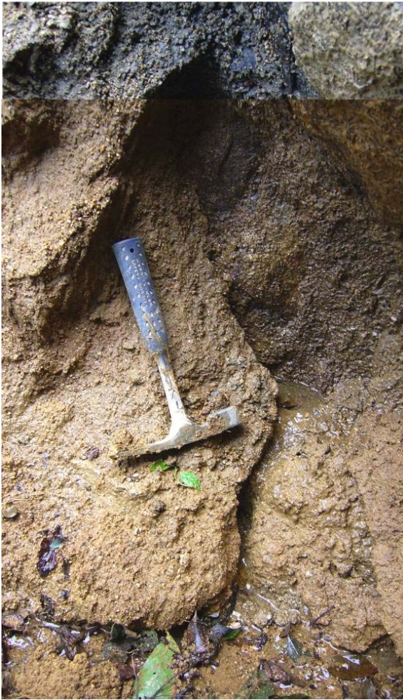
Plate 16 - Active Seepage from Sandy Joint Infill of Main Scarp (Photograph taken on 29 August 2005)
