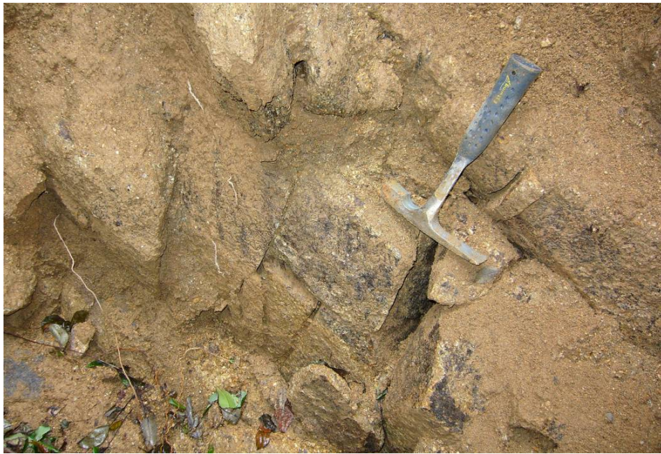
Plate 10 - Close-up View of Main Scarp of Retrogressive Area Showing Distinct Block Displacement and Joint Opening (Photograph taken on 29 August 2005)
