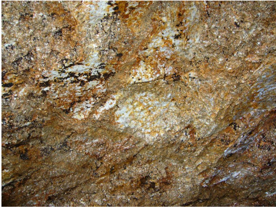
Plate 12 - Kaolinisation of Grade V Granite in the Eastern Flank (Photograph taken on 29 August 2005)
