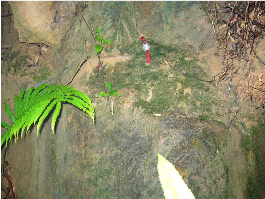
Plate 29 - Exposure of Moderately Decomposed Granite Rock Upslope (Southwest) of Landslide Source (Located west of the exposure in Plate 28, Photograph taken on 25 August 2005)
