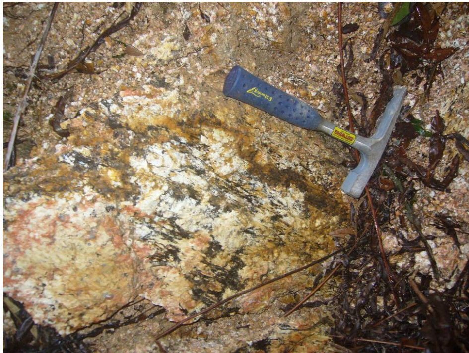
Plate 28 - Exposure Upslope (Southwest) of Landslide Source, Showing Decomposed Granite, Kaolinisation and Slickensides (Photograph taken on 25 August 2005)
